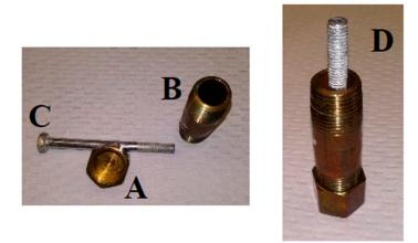
**Figure S3.** The bone crusher was made using three components. The bottom part (**A**) screws on to the barrel (**B**). The piston (**C**) then can be used to pulverize the bone using a hammer. (**D**) is the finished crusher.
