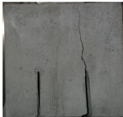
**Figure 12.** Characteristic crack path observed in the tests.
