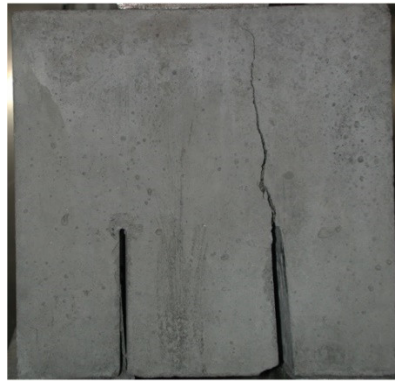
Figure 12. Characteristic crack path observed in the tests.
