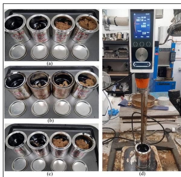
**Figure 6.** (a) Bitumen C170, (b) Bitumen A10E, (c) Bitumen C320, and (d) blending of bitumen with fibers using the shear mixture.
