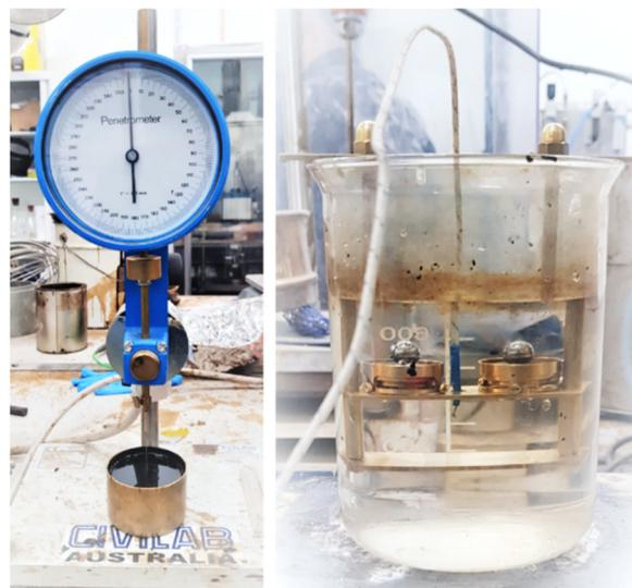
**Figure 8.** Penetration test (on left) and softening point test (on right) of a sample carried out in this study.
