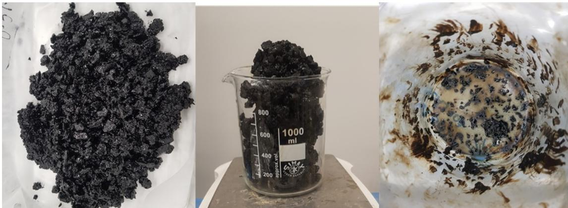
**Figure 16.** Binder drain off process. Asphalt mix prepared with CBs modified bitumen (**left**); preparation of binder drain off test (**middle**); drained off binder with fine aggregates retained at the bottom of glass flask (**right**).
