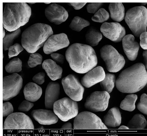
**Figure 1.** Grains of quartz sand.
