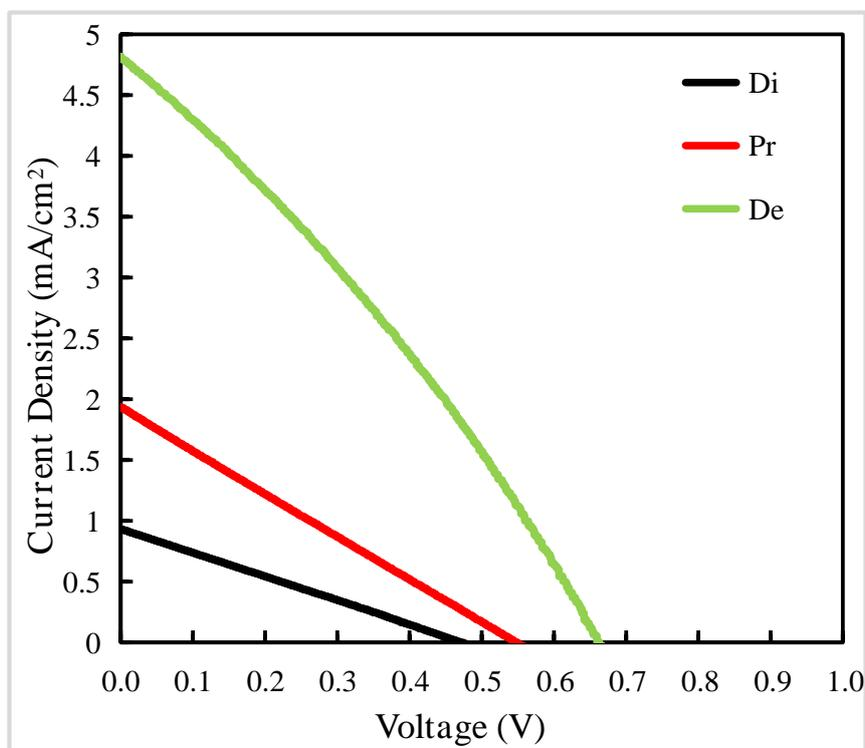
**Figure 3.** Reverse scanning J–V curves of PSCs based on Process 1. The letter Di, Pr, De represent films prepared with Direct method, Proportional method, and Delayed method, respectively. The device active area is 0.25 cm<sup>2</sup> (0.5 cm × 0.5 cm). The meaning of Process 1, Direct method, Proportional method and Delayed method is described in the second paragraph of experimental Section 2.2.2.
