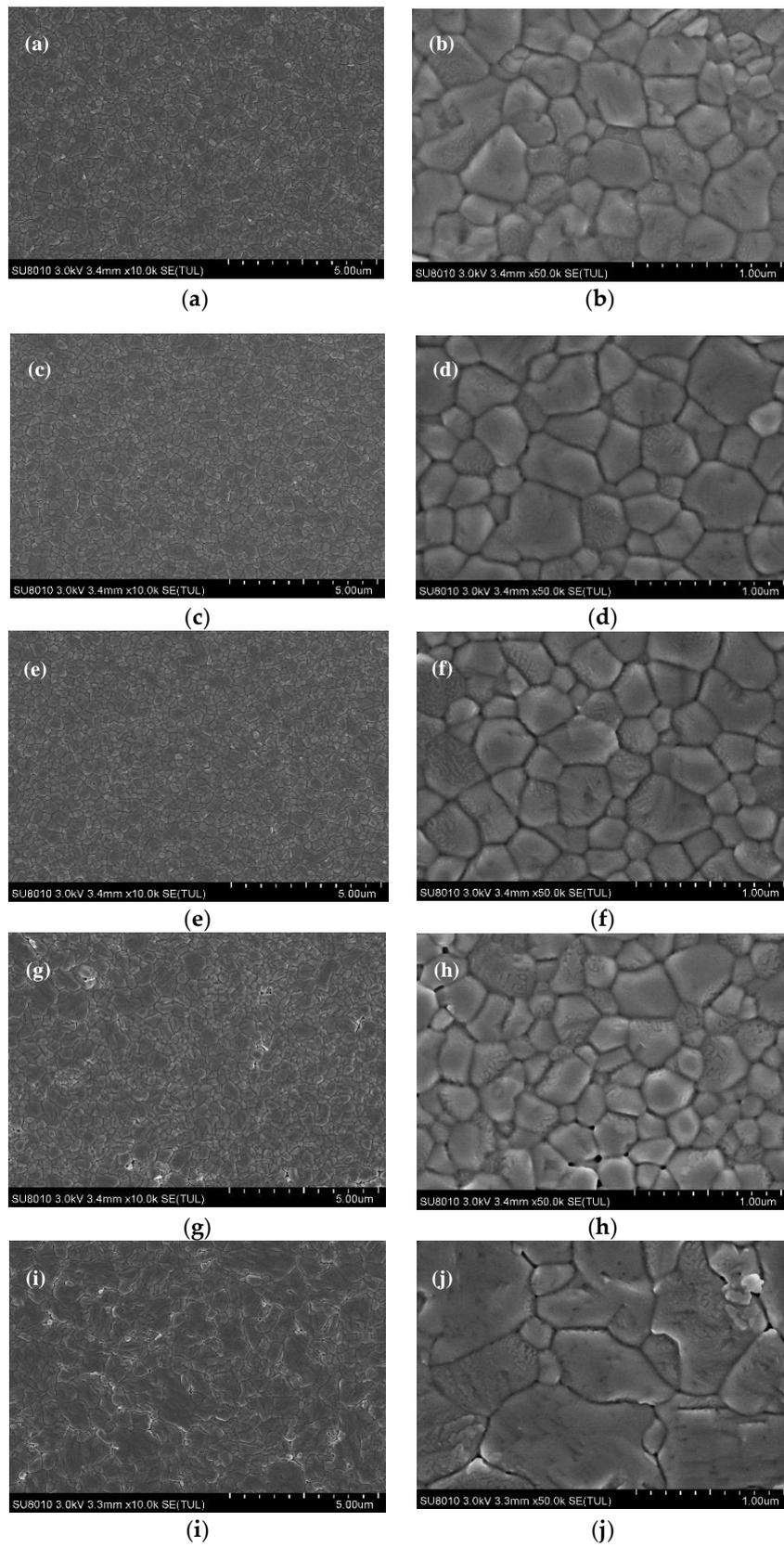
**Figure 5.** SEM images of perovskite film prepared on nano  $\text{TiO}_2$  optimized with (6,6)-phenyl  $\text{C}_{61}$  butyric acid methyl ester ( $\text{PC}_{61}\text{BM}$ ) of different concentration: (a,c,e,g,i) The low magnification; (b,d,f,h,j) The high magnification.
