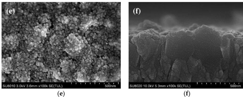
**Figure 2.** Scanning electron microscope (SEM) images of nano TiO<sub>2</sub> films using Process 1: (a,c,e) The top-view images under Direct method, Proportional method, and Delayed method, respectively; (b,d,f) The corresponding cross-sectional images. The meaning of Process 1, Direct method, Proportional method and Delayed method is described in the second paragraph of experimental Section 2.2.2.
