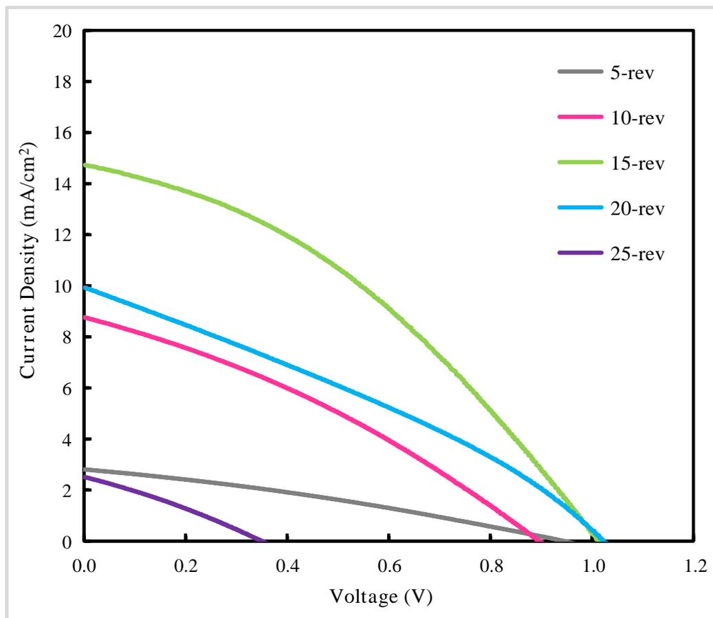
**Figure 8.** Reverse scanning J–V curves of perovskite solar cells optimized with different concentration of PC<sub>61</sub>BM. -rev represents reverse scanning. The number 5, 10, 15, 20, 25 represent different concentration of PC<sub>61</sub>BM. The device active area is 0.25 cm<sup>2</sup> (0.5 cm × 0.5 cm).
