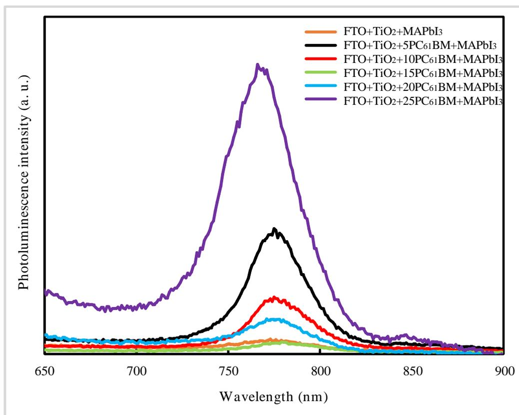
**Figure 7.** Photoluminescence spectra of perovskite films deposited on PC<sub>61</sub>BM of different concentration. The number 5, 10, 15, 20, 25 represent different concentration of PC<sub>61</sub>BM.
