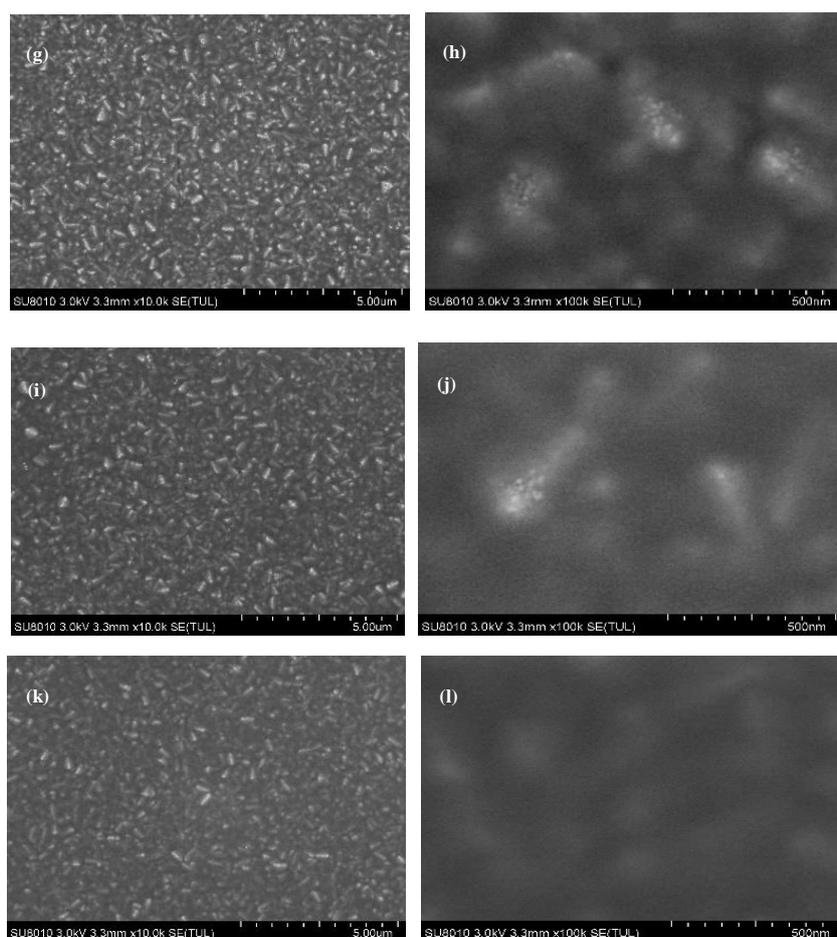
**Figure 4.** SEM images of nano  $\text{TiO}_2$  layer under Process 2: (a,c,e,g,i,k) Represent 0, 5, 10, 15, 20, 25 mg/mL, respectively, the low magnification; (b,d,f,h,j,l) The corresponding high magnification. The meaning of Process 2 is described in the third paragraph of experimental Section 2.2.2.
