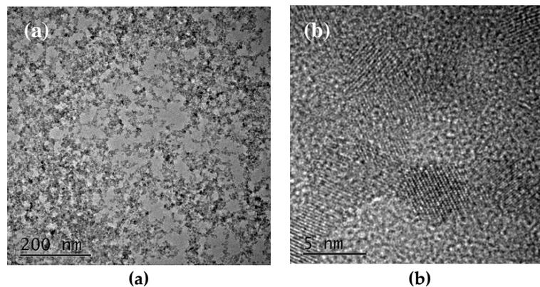
**Figure 1.** Transmission electron microscope (TEM) images of  $\text{TiO}_2$  nanoparticles: (a) The low magnification; (b) The high magnification.
