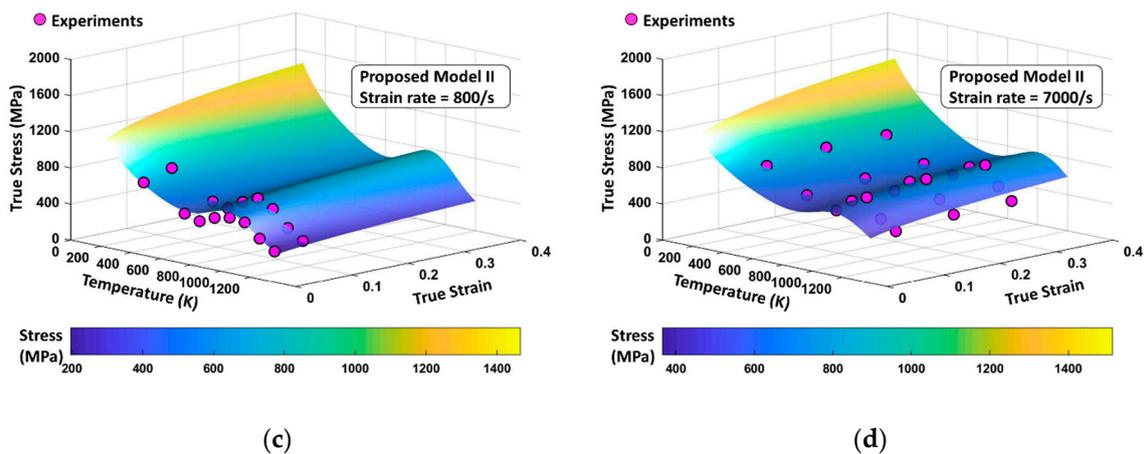
**Figure 24.** The PM II flow stress surfaces according to variation of temperature and strain level with (a)  $\dot{\epsilon} = 0.001 \text{ s}^{-1}$ , (b)  $\dot{\epsilon} = 0.02 \text{ s}^{-1}$ , (c)  $\dot{\epsilon} = 800 \text{ s}^{-1}$ , and (d)  $\dot{\epsilon} = 7000 \text{ s}^{-1}$ . The experimental data are from [1].
