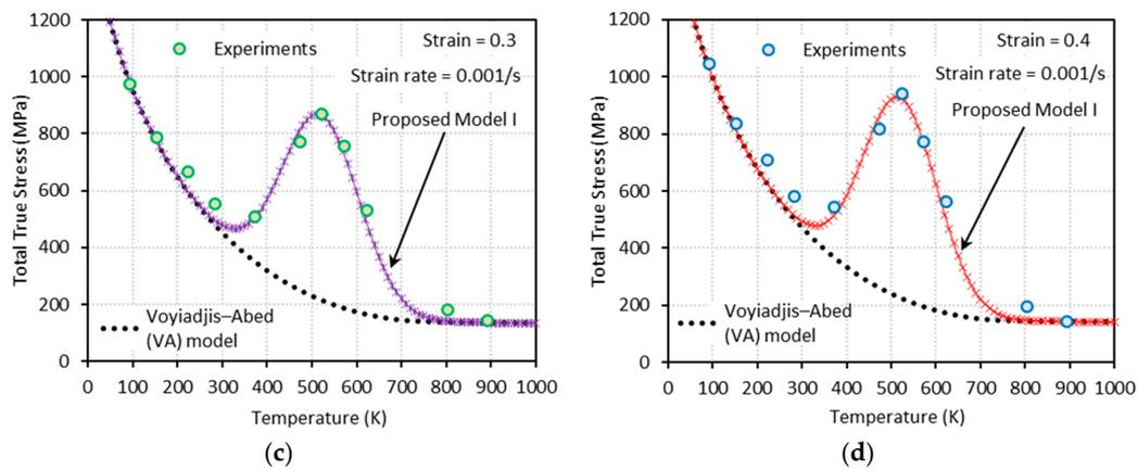
**Figure 9.** Comparisons between model predictions from the VA and proposed model I and experimental data from [1] on the total true stress versus temperature responses at (a)  $\epsilon = 0.1$ , (b)  $\epsilon = 0.2$ , (c)  $\epsilon = 0.3$ , and (d)  $\epsilon = 0.4$ . Quasi-static loading with  $\dot{\epsilon} = 0.001 \text{ s}^{-1}$  is applied.
