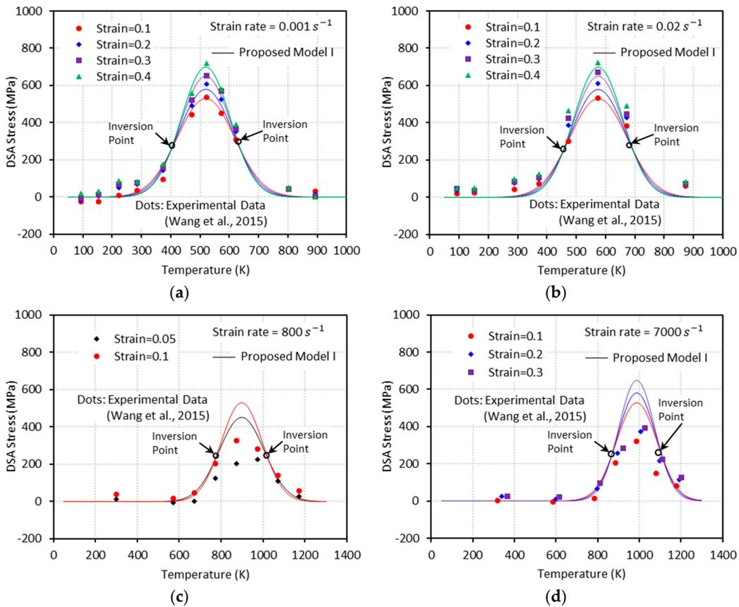
**Figure 8.** The DSA-induced flow stress versus temperature curves from the experiments [1] and the proposed model I with (a)  $\dot{\epsilon} = 0.001 \text{ s}^{-1}$ , (b)  $\dot{\epsilon} = 0.02 \text{ s}^{-1}$ , (c)  $\dot{\epsilon} = 800 \text{ s}^{-1}$ , and (d)  $\dot{\epsilon} = 7000 \text{ s}^{-1}$ .
