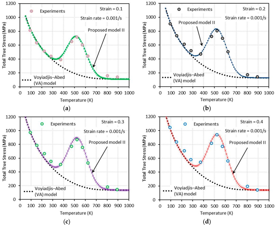
**Figure 14.** Comparisons between model predictions from the VA and proposed model II and experimental data from [1] on the total true stress versus temperature responses at (a)  $\epsilon = 0.1$ , (b)  $\epsilon = 0.2$ , (c)  $\epsilon = 0.3$ , and (d)  $\epsilon = 0.4$ . Quasi-static loading with  $\dot{\epsilon} = 0.001 \text{ s}^{-1}$  is applied.
