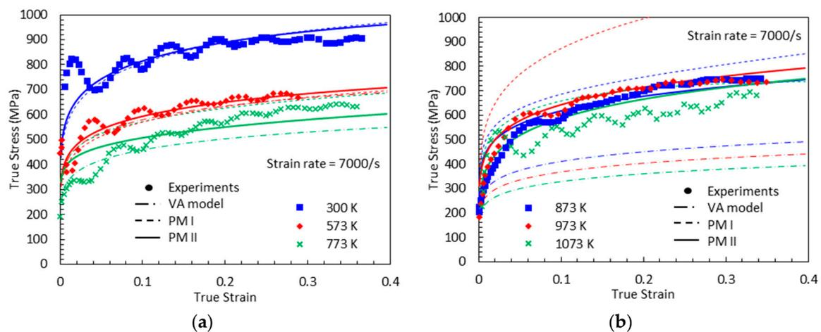
**Figure 22.** True stress-true strain curves from experimental measurement [1], predictions by the VA model, PM I, and PM II with  $\dot{\epsilon} = 7000 \text{ s}^{-1}$ : (a)  $T = 300, 573$  and  $773 \text{ K}$  (b)  $T = 873, 973$  and  $1073 \text{ K}$ .
