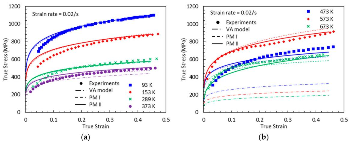
**Figure 20.** True stress-true strain curves from experimental measurement [1], predictions by the VA model, PM I, and PM II with  $\dot{\epsilon} = 0.02 \text{ s}^{-1}$ : (a)  $T = 93, 153, 289$  and  $373 \text{ K}$  (b)  $T = 473, 573$  and  $673 \text{ K}$ .
