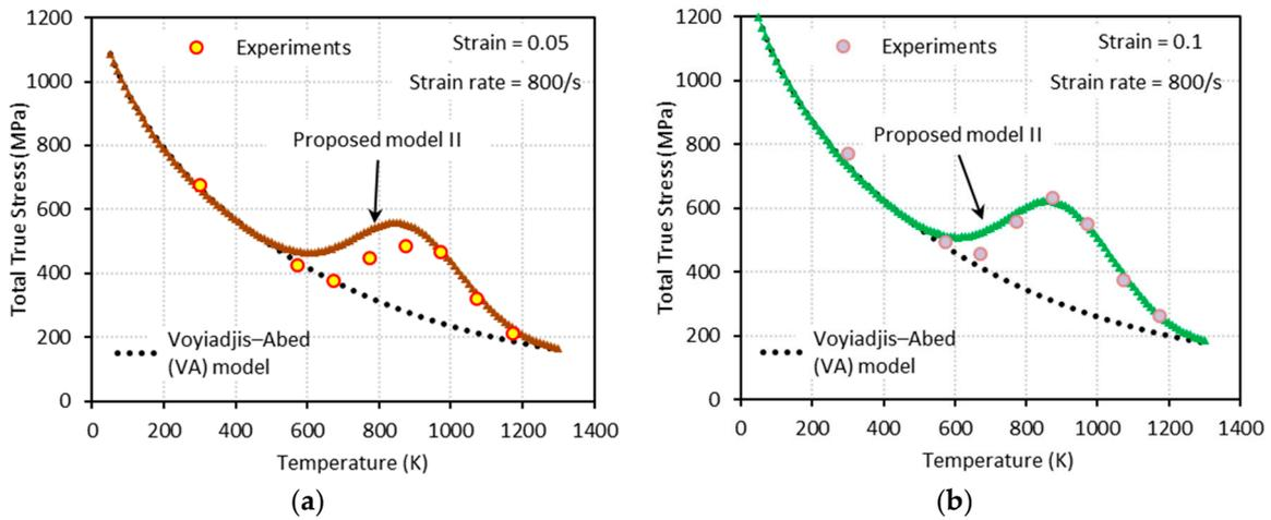
**Figure 16.** Comparisons between model predictions from the VA and proposed model II and experimental data from [1] on the total true stress versus temperature responses at (a)  $\epsilon = 0.05$  and (b)  $\epsilon = 0.1$ . Dynamic loading with  $\dot{\epsilon} = 800 \text{ s}^{-1}$  is applied.
