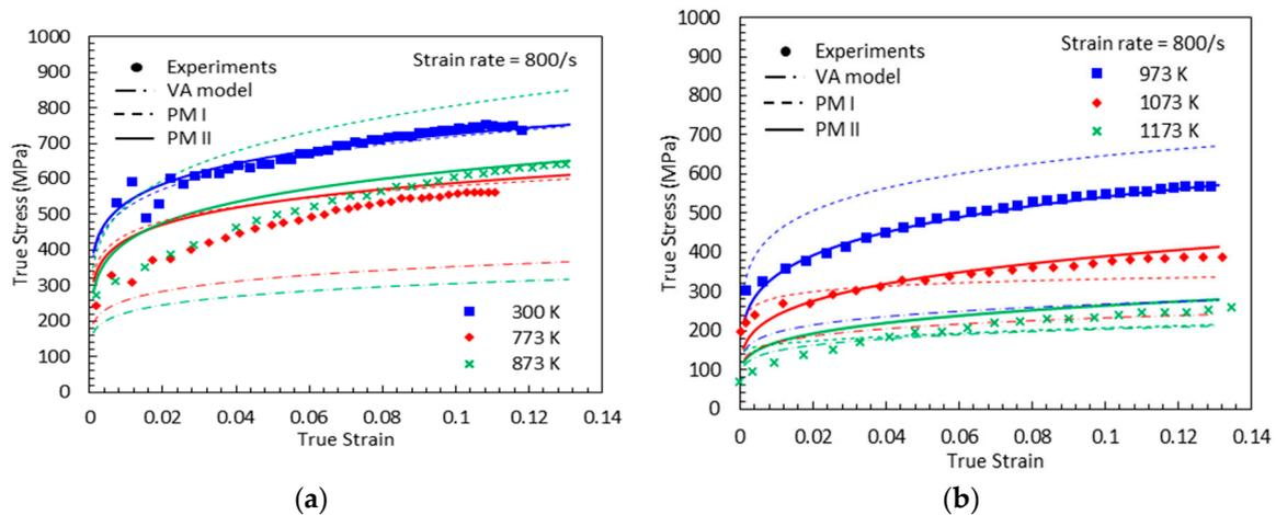
**Figure 21.** True stress-true strain curves from experimental measurement [1], predictions by the VA model, PM I, and PM II with  $\dot{\epsilon} = 800 \text{ s}^{-1}$ : (a)  $T = 300, 773$  and  $873 \text{ K}$  (b)  $T = 973, 1073$  and  $1173 \text{ K}$ .
