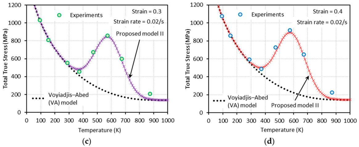
**Figure 15.** Comparisons between model predictions from the VA and proposed model II and experimental data from [1] on the total true stress versus temperature responses at (a)  $\epsilon = 0.1$ , (b)  $\epsilon = 0.2$ , (c)  $\epsilon = 0.3$ , and (d)  $\epsilon = 0.4$ . Quasi-static loading with  $\dot{\epsilon} = 0.02 \text{ s}^{-1}$  is applied.
