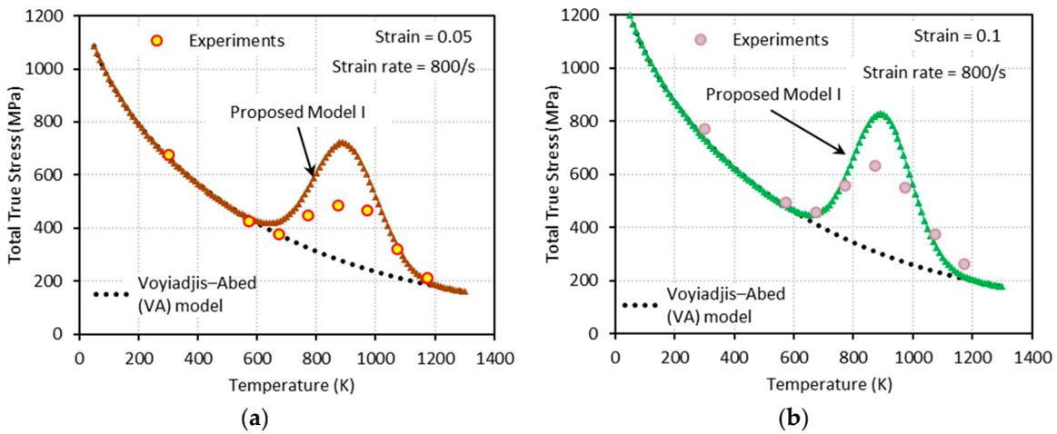
**Figure 11.** Comparisons between model predictions from the VA and proposed model I and experimental data from [1] on the total true stress versus temperature responses at (a)  $\epsilon = 0.05$  and (b)  $\epsilon = 0.1$ . Dynamic loading with  $\dot{\epsilon} = 800 \text{ s}^{-1}$  is applied.
