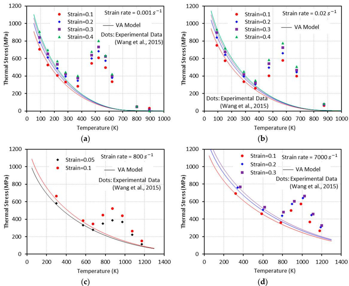
**Figure 5.** The thermal flow stress versus temperature curves from the experiments [1] and the VA model (Equation (15)) with (a)  $\dot{\epsilon} = 0.001 \text{ s}^{-1}$ , (b)  $\dot{\epsilon} = 0.02 \text{ s}^{-1}$ , (c)  $\dot{\epsilon} = 800 \text{ s}^{-1}$ , and (d)  $\dot{\epsilon} = 7000 \text{ s}^{-1}$ .
