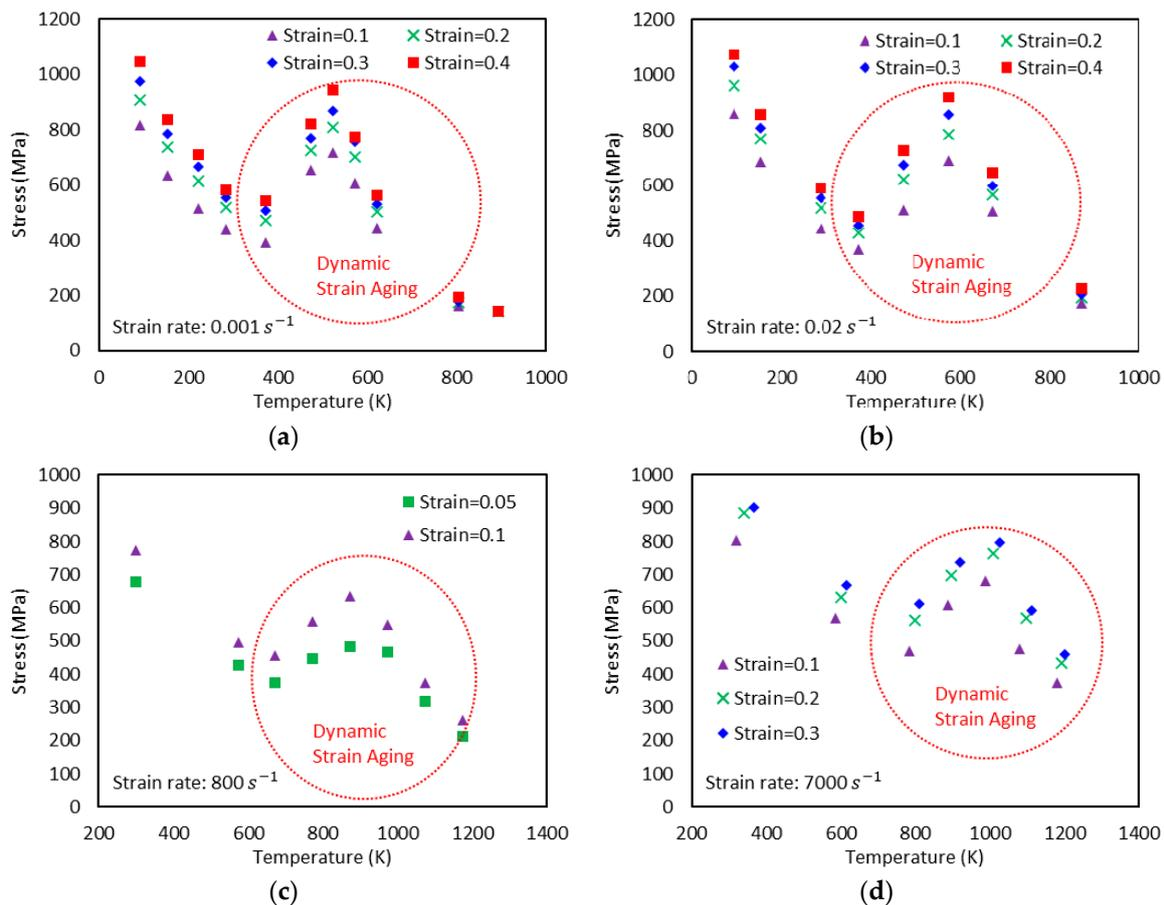
**Figure 1.** Experimental stress-temperature graphs for Q235B steel for different strain rates ( $\dot{\epsilon}$ ) and strain levels: (a)  $\dot{\epsilon} = 0.001\text{ s}^{-1}$ , (b)  $\dot{\epsilon} = 0.02\text{ s}^{-1}$ , (c)  $\dot{\epsilon} = 800\text{ s}^{-1}$ , and (d)  $\dot{\epsilon} = 7000\text{ s}^{-1}$  [1]. Dynamic strain aging (DSA) is observed in all cases.
