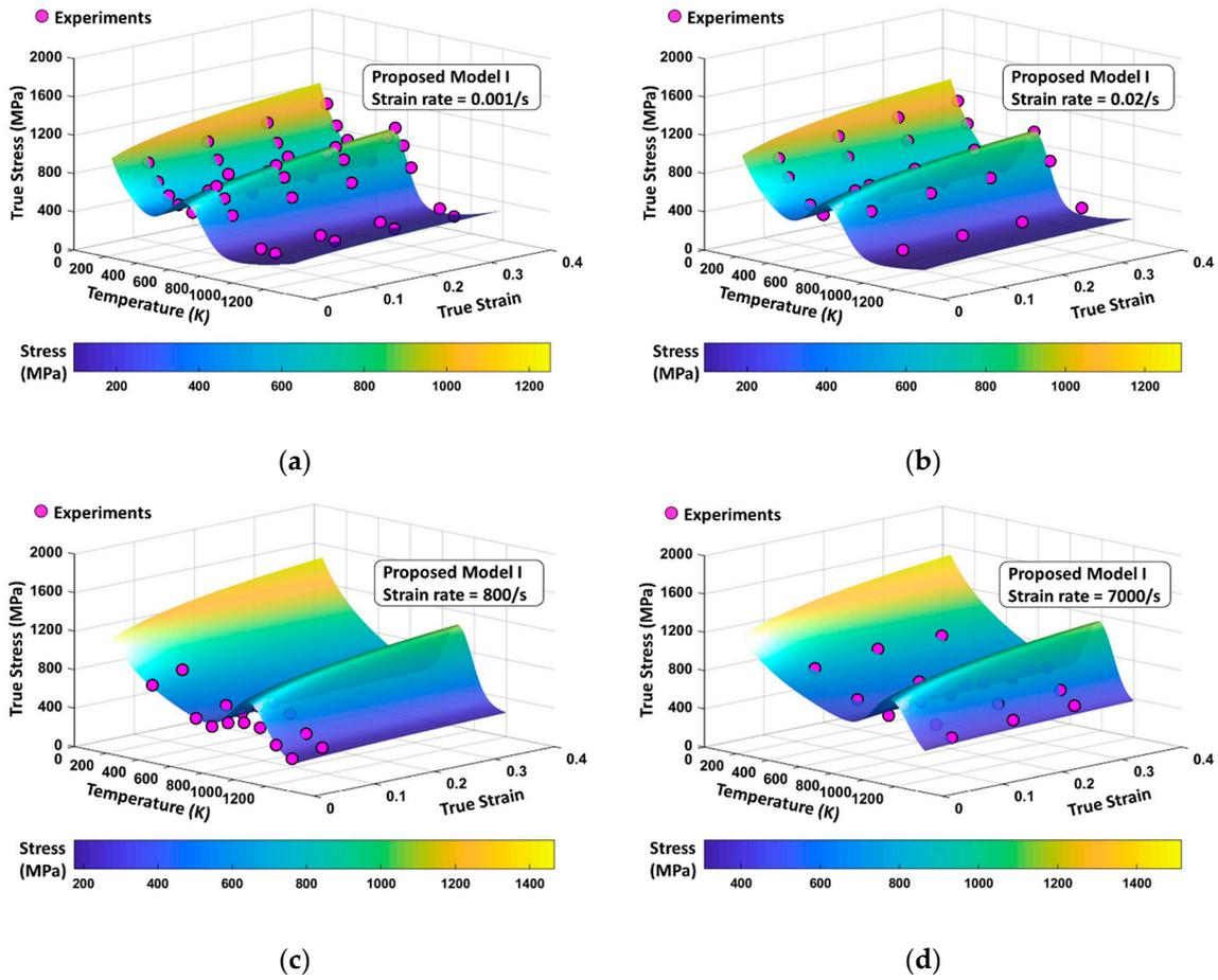
**Figure 23.** PM I flow stress surfaces according to variation of temperature and strain level with (a)  $\dot{\epsilon} = 0.001 \text{ s}^{-1}$ , (b)  $\dot{\epsilon} = 0.02 \text{ s}^{-1}$ , (c)  $\dot{\epsilon} = 800 \text{ s}^{-1}$ , and (d)  $\dot{\epsilon} = 7000 \text{ s}^{-1}$ . The experimental data are from [1].
