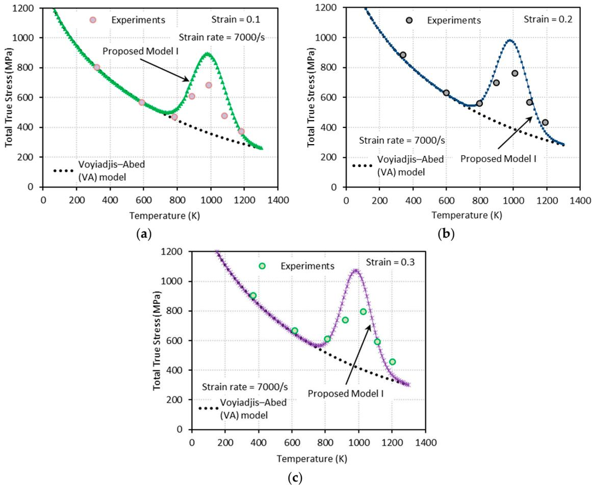
**Figure 12.** Comparisons between model predictions from the VA and proposed model I and experimental data from [1] on the total true stress versus temperature responses at (a)  $\epsilon = 0.1$ , (b)  $\epsilon = 0.2$ , and (c)  $\epsilon = 0.3$ . Dynamic loading with  $\dot{\epsilon} = 7000 \text{ s}^{-1}$  is applied.
