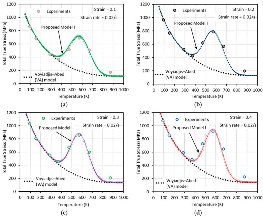
**Figure 10.** Comparisons between model predictions from the VA and proposed model I and experimental data from [1] on the total true stress versus temperature responses at (a)  $\epsilon = 0.1$ , (b)  $\epsilon = 0.2$ , (c)  $\epsilon = 0.3$ , and (d)  $\epsilon = 0.4$ . Quasi-static loading with  $\dot{\epsilon} = 0.02 \text{ s}^{-1}$  is applied.
