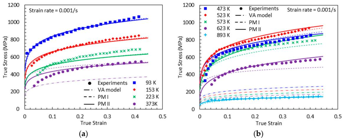
**Figure 19.** True stress-true strain curves from experimental measurement [1], predictions by the VA model, proposed model (PM) I, and PM II with  $\dot{\epsilon} = 0.001 \text{ s}^{-1}$ : (a)  $T = 93, 153, 223$  and  $373 \text{ K}$  (b)  $T = 473, 523, 573, 623$  and  $893 \text{ K}$ .
