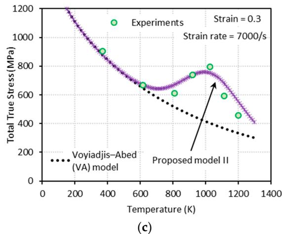
**Figure 17.** Comparisons between model predictions from the VA and proposed model II and experimental data from [1] on the total true stress versus temperature responses at (a)  $\epsilon = 0.1$ , (b)  $\epsilon = 0.2$ , and (c)  $\epsilon = 0.3$ . Dynamic loading with  $\dot{\epsilon} = 7000 \text{ s}^{-1}$  is applied.
