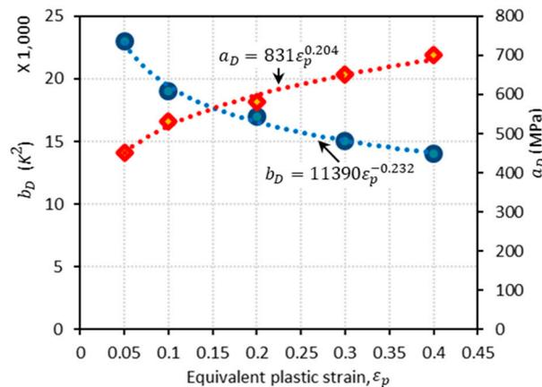
**Figure 6.** The plots of  $a_D$  and  $b_D$  versus  $\varepsilon_p$ . Dots for both of the parameters are obtained from the experimental data [1]. The corresponding trend lines are displayed using a power law form.
