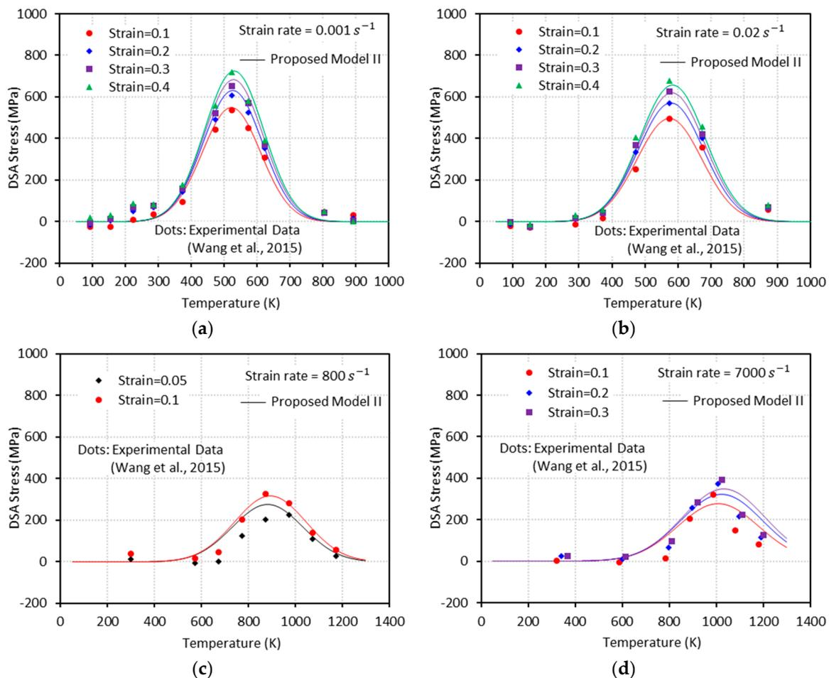
**Figure 13.** The DSA-induced flow stress versus temperature curves from the experiments [1] and the proposed model II with (a)  $\dot{\epsilon} = 0.001 s^{-1}$ , (b)  $\dot{\epsilon} = 0.02 s^{-1}$ , (c)  $\dot{\epsilon} = 800 s^{-1}$ , and (d)  $\dot{\epsilon} = 7000 s^{-1}$ .
