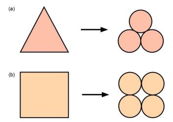
**Figure 3.** Illustration of clump formation: (**a**) Triangular particle made from nine overlapping circular particles and (**b**) Square particle made from 15 overlapping circular particles.
