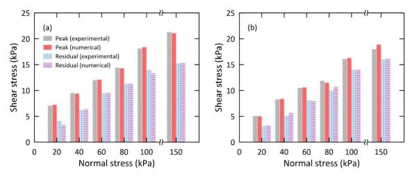
Figure 7. Shear stress vs. normal stress: (a) drained and (b) undrained condition.
