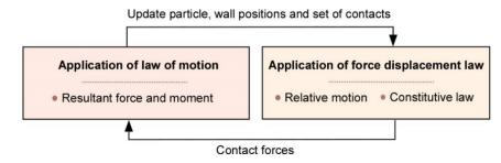
Figure 2. Discrete Element Method (DEM) computational scheme in PFC<sup>2D.</sup>
