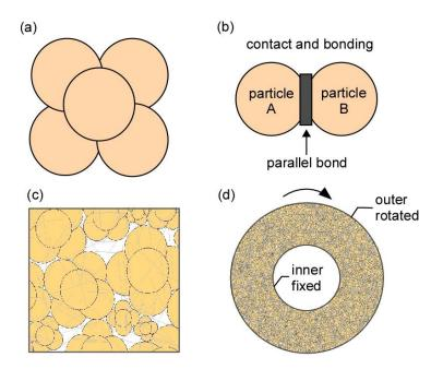
**Figure 4.** Clump particles and assembly: (**a**) clump particle, (**b**) parallel bond idealization between particles, (**c**) parallel bond connection between clump particles and (**d**) clump particles in ring shear box.
