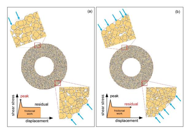
**Figure 10.** Clump particle crushing at: (**a**) peak shear stress and (**b**) residual shear stress. Arrows indicate a progressive occurrence of clump particle crushing.
