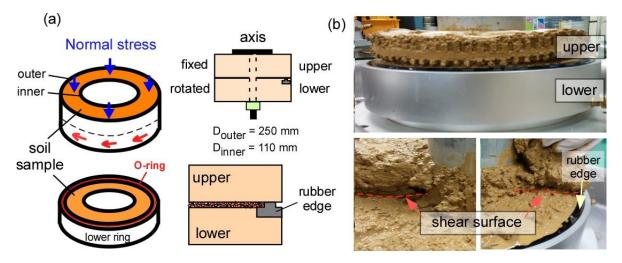
**Figure 1.** Schematical illustration of the ring shear box and shear surface after testing: (**a**) configuration of ring shear box and (**b**) observation of shear surface after testing.
