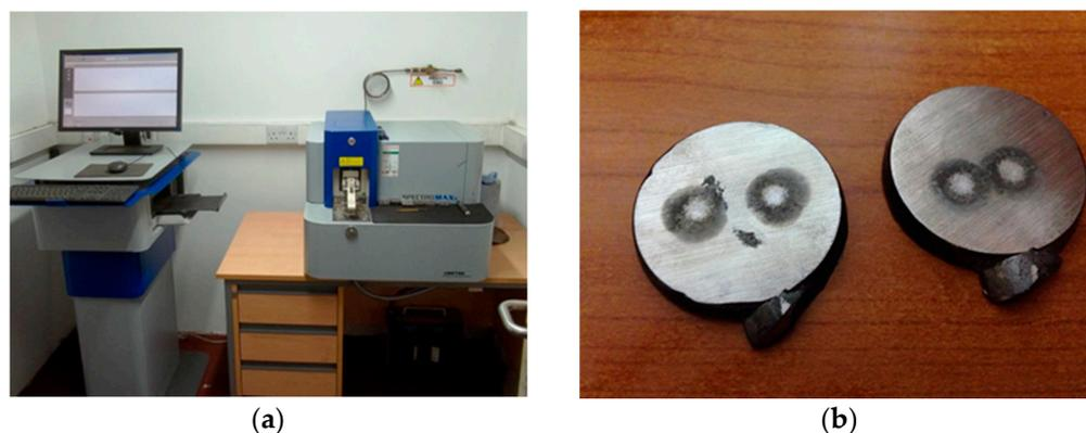
**Figure 7.** Equipment and samples used for chemical analysis (a) the SPECTROMAXx chemical analysis spectrometer of Benninger Guss AG. (b) Surface of the samples after chemical analysis performed with the spectrometer.
