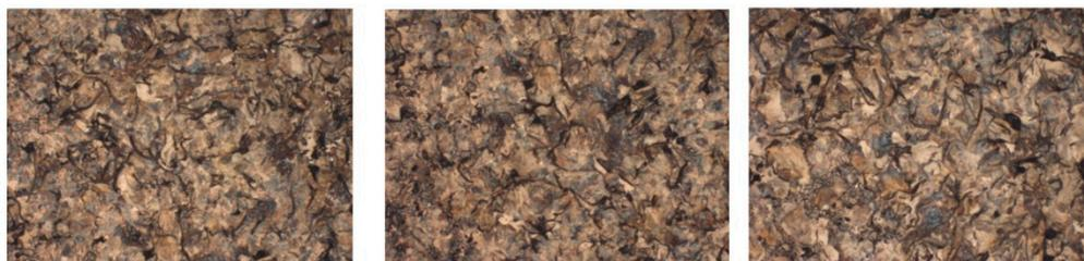
**Figure 20.** Microstructure of cast iron samples with lamellar graphite type EN-GJL-250, after metallographic attack at 100× magnification.
