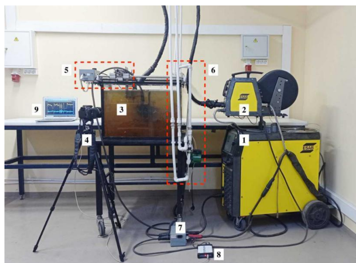
Figure 1. Underwater wet cutting setup: (1) source of power; (2) wire feed system; (3) water tank; (4) video camera; (5) automat of torch movement; (6) water supply system and pump; (7) welding current and arc voltage sensors; (8) USB-oscilloscope; (9) laptop.
