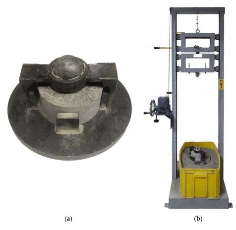
Figure 3. Free-fall impact test: (a) test equipment and KFRC specimen; (b) test machine.
