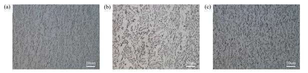
Figure 4. OM images on 1/4 length sections of E36 (a), EH36 (b) and FH36 (c) steel plates.
