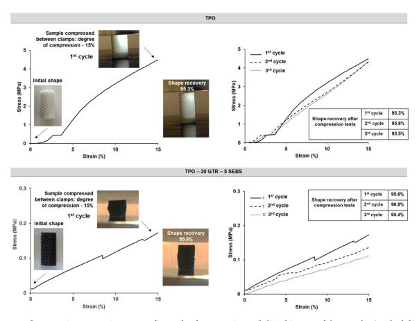
**Figure 12.** Stress–strain compression curves: first cycle of compression and digital images of the samples (on the left) and reproducibility of the compression tests (three successive fatigue cycle tests; on the right) of TPO and TPO-30 GTR-5 SEBS samples.
