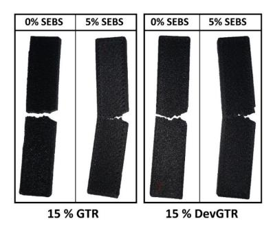
**Figure 6.** Images of ABS impact specimens (after test), containing 15 wt.% GTR or DevGTR, with and without the incorporation of SEBS (5 wt.%).
