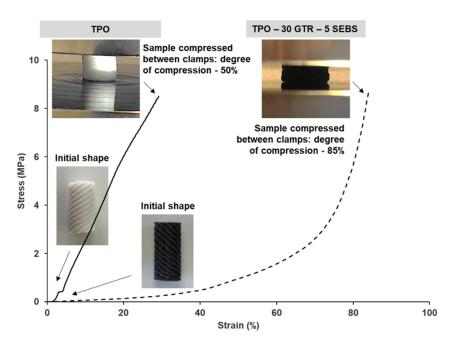
Figure 11. Stress-strain compression curves for TPO and TPO-30 GTR-5 SEBS samples.
