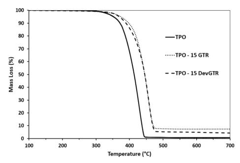
Figure 7. TGA thermograms of TPO, TPO-GTR, and TPO-DevGTR materials (under  $N_2$ , 10  $^{\circ}$ C/min).
