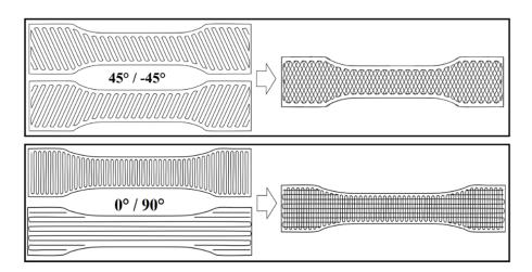
**Figure 3.** Schematic presentation of the raster angle  $45^{\circ}/-45^{\circ}$  and  $0^{\circ}/90^{\circ}$  used for the ABS-based samples 3D printing.
