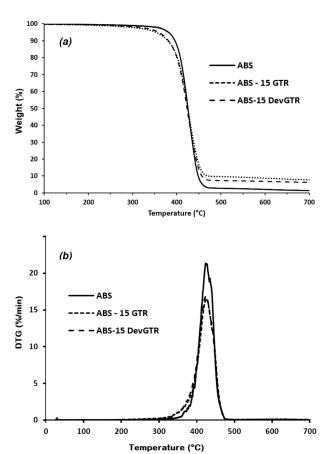
**Figure 4.** TGA (a) and DTG (b) thermograms of ABS-based composites (under  $N_2$ , 10 °C/min).
