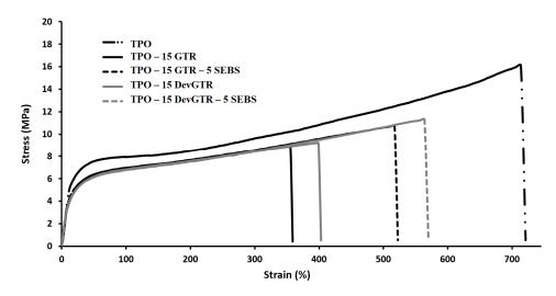
Figure 8. Stress-strain curves of TPO and TPO-recycled tire rubber blends as prepared by 3D printing.
