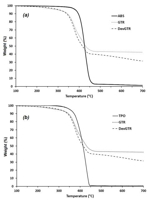
**Figure 2.** TGA thermograms of vulcanized (GTR), devulcanized (DevGTR) recycled tire rubber powders and ABS (**a**) and TPO (**b**) (under  $N_2$ , 10 °C/min).
