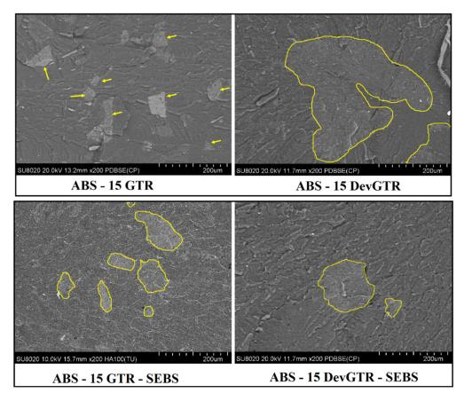
**Figure 5.** SEM micrographs of ABS-based materials containing GTR or DevGTR with or without the addition of SEBS.
