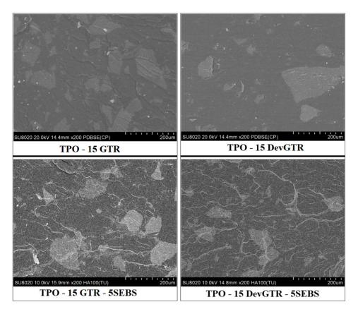
**Figure 10.** SEM micrographs of TPO containing 15 wt.% GTR or DevGTR, with or without the incorporation of 5 wt.% SEBS.
