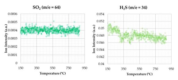
Figure 9. SO<sub>2</sub> and H<sub>2</sub>S emissions (oxidizing atmosphere).
