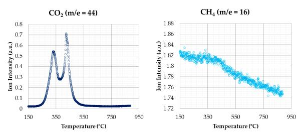
Figure 7. CO<sub>2</sub> and CH<sub>4</sub> emissions (oxidizing atmosphere).
