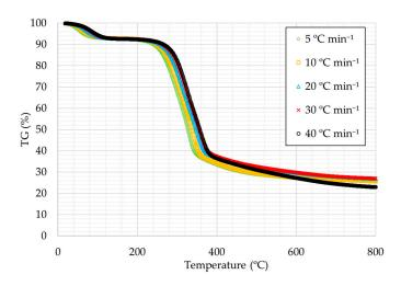
Figure 2. TG curves for the heating rates studied under inert atmosphere.
