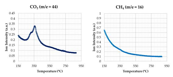
Figure 10. CO<sub>2</sub> and CH<sub>4</sub> emissions (inert atmosphere).
