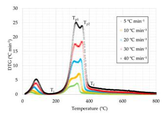
Figure 4. DTG curves for the heating rates studied under inert atmosphere.
