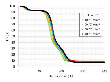
Figure 1. TG curves for the heating rates studied under oxidative atmosphere.
