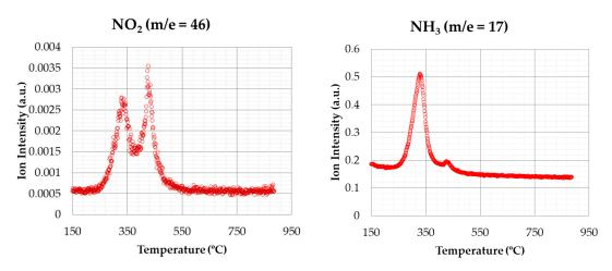
Figure 8. NO<sub>2</sub> and NH<sub>3</sub> emissions (oxidizing atmosphere).
