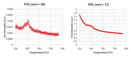
Figure 11. NO<sub>2</sub> and NH<sub>3</sub> emissions (inert atmosphere).
