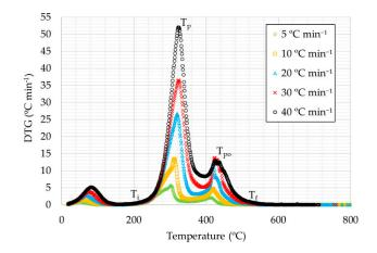
Figure 3. DTG curves for the heating rates studied under oxidative atmosphere.
