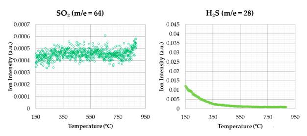
Figure 12. SO<sub>2</sub> and H<sub>2</sub>S emissions (inert atmosphere).
