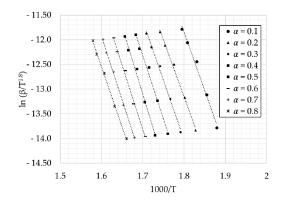
Figure 5. FWO, KAS, and Starink plots for the values of conversion degree.
