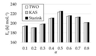
**Figure 6.** Activation energy obtained by FWO, KAS, and Starink methods, at different conversion rates.
