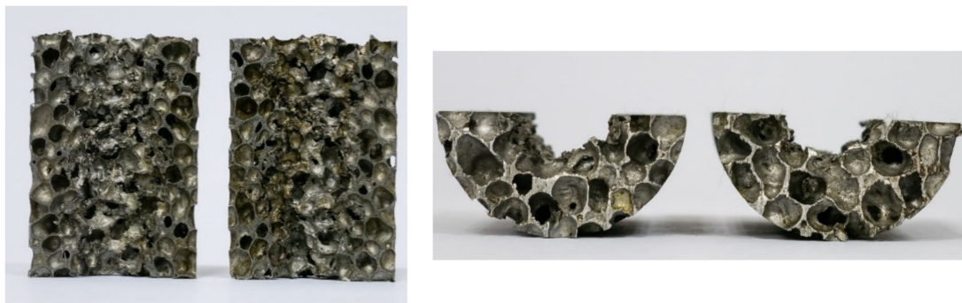
Figure 15. Cutting image of trajectories of steel balls penetrating aluminum foam.
