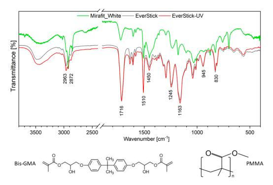
**Figure 6.** Fourier-transformed mid-infrared spectra of neat EverStick post, UV light-cured EverStick post, Mirafit White and GC Fibre post (**top**) and the structural formula of bisphenol A–glycidyl methacrylate (bis–GMA) (**bottom left**) and poly (methyl methacrylate) PMMA (**bottom right**).
