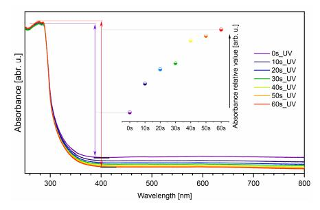
**Figure 7.** Absorption spectra of neat EverStick post and UV light-cured EverStick post as a function of light-curing time. Inset—The amplitude between the maximum and minimum absorption value.
