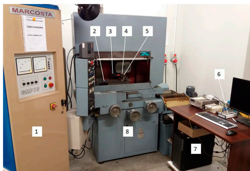
Figure 1. Test stand: 1—electro-spark discharge generator, 2—electric voltage supply to the working electrode, 3—dielectric liquid nozzle, 4—grinding wheel, 5—working electrode, 6—card terminal, 7—PC computer, 8—ECBT8 grinder.
