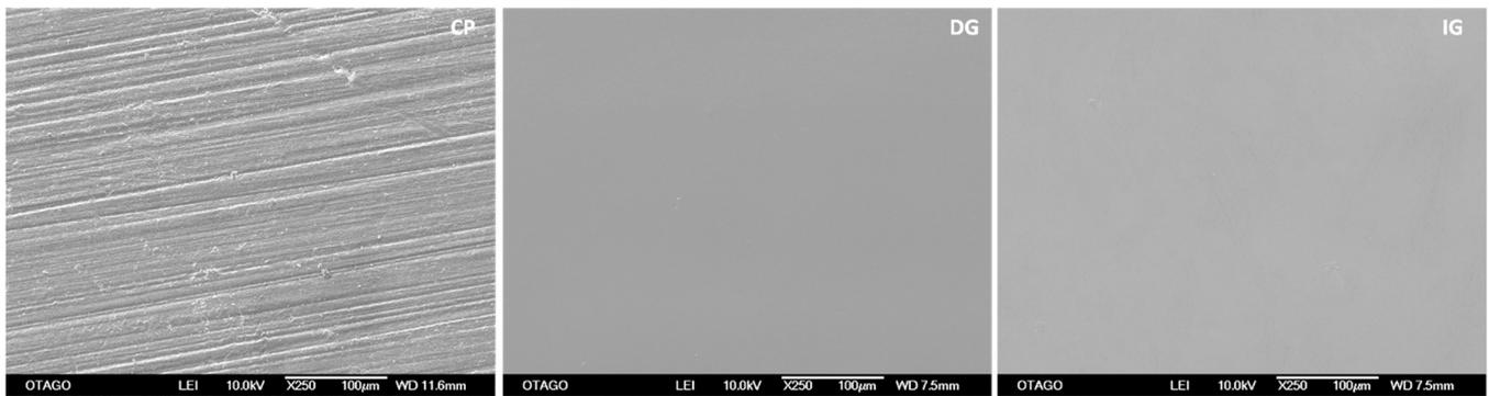
**Figure 3.** SEM images showing surface texture at 250 $\times$  (group CP, DG and IG). Note the nonglazed surface appear rougher compared to glazed surfaces.
