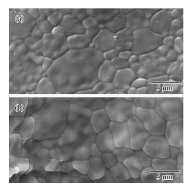
**Figure 10.** Ceramic microstructures in alumina crowns. Crystal grains observed by the scanning electron microscopy (SEM). Cross sections of the (**a**) horizontal and (**b**) vertical planes are defined as the parallel and vertical views of the laminated layers.
