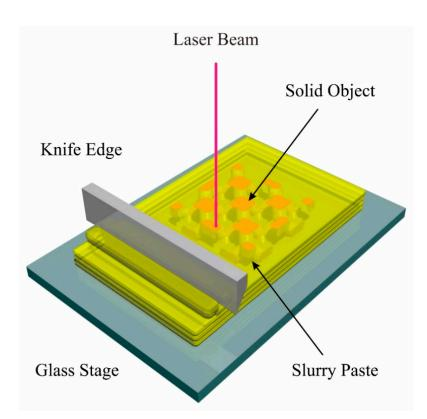
**Figure 1.** Schematic illustration of stereolithographic additive manufacturing (STL-AM). Crosssectional layers are formed on paste materials by laser scanning. Solid objects are fabricated via layer laminating and interlayer bonding.
