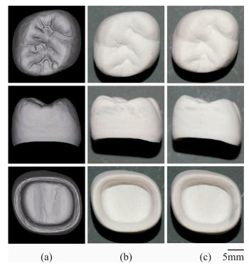
**Figure 9.** Dental crowns fabricated by STL-AM. Top and side views of the graphic model (**a**); composite precursor (**b**), and ceramic component (**c**) arranged in the same magnification.
