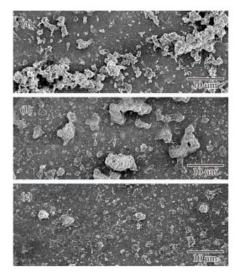
**Figure 6.** Alumina particles dispersed in acrylic resin. Paste containers were rotated and revolved for processing times of 300, 600, and 900 s. Cross sections of solid films are shown in (**a**–**c**).
