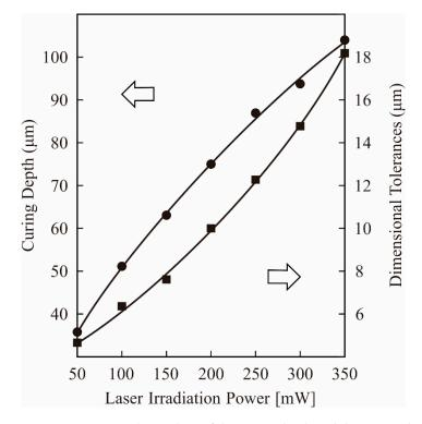
**Figure 8.** Corresponding values of the curing depth and dimensional tolerances for laser irradiation powers. Layer thickness and hole diameters were measured in the film specimens, as shown in Figure 2.
