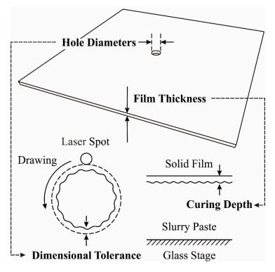
**Figure 2.** Drawing pattern of film specimens to optimize lithographic conditions. Hole diameters and layer thicknesses were measured by a digital optical microscope. Dimensional tolerances and curing depth were estimated.
