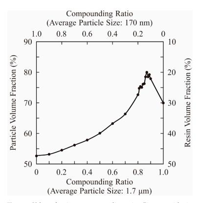
**Figure 3.** Volume fractions at compounding ratios. Binary particle sizes of 170 nm and 1.7  $\mu$ m in diameters were adjusted. Closed packs of spherical fillers were simulated by a distinct element method (DEM).
