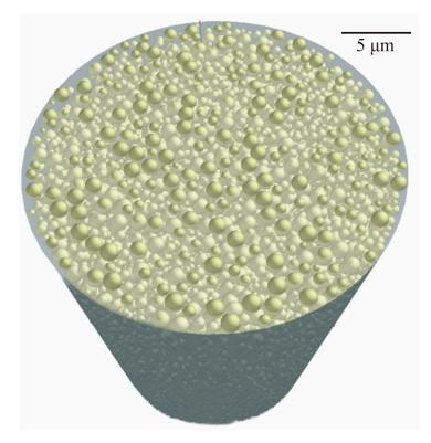
**Figure 4.** Dispersion profiles of bimodal powders in resin matrixes. Maximum contents were optimized at 80% of the total volume fraction. Computer graphics were plotted according to the DEM simulations.
