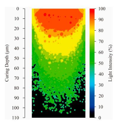
**Figure 5.** Intensity profile of optical irradiation at the laser spot. Vertical sections of polymerized regions were visualized. Ultraviolet (UV) light propagation in the particles gaps was simulated by the ray tracing (RT) method.
