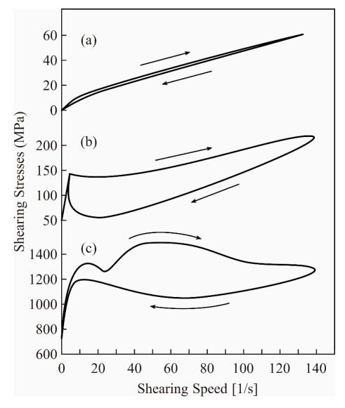
**Figure 7.** Dynamic profiles of shearing stresses and speeds. Rheological profiles were analyzed by a kinematic viscometer (KV). Viscose pastes processed for 300, 600, and 900 s are shown in (**a**–**c**), respectively.
