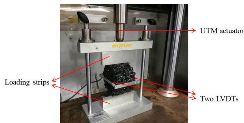
**Figure 2.** ITT fatigue test.
