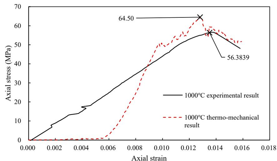
**Figure 5.** Comparison of experimental and predicted stress–strain relationships for rocks subjected to heat treatment at 1000 °C.
