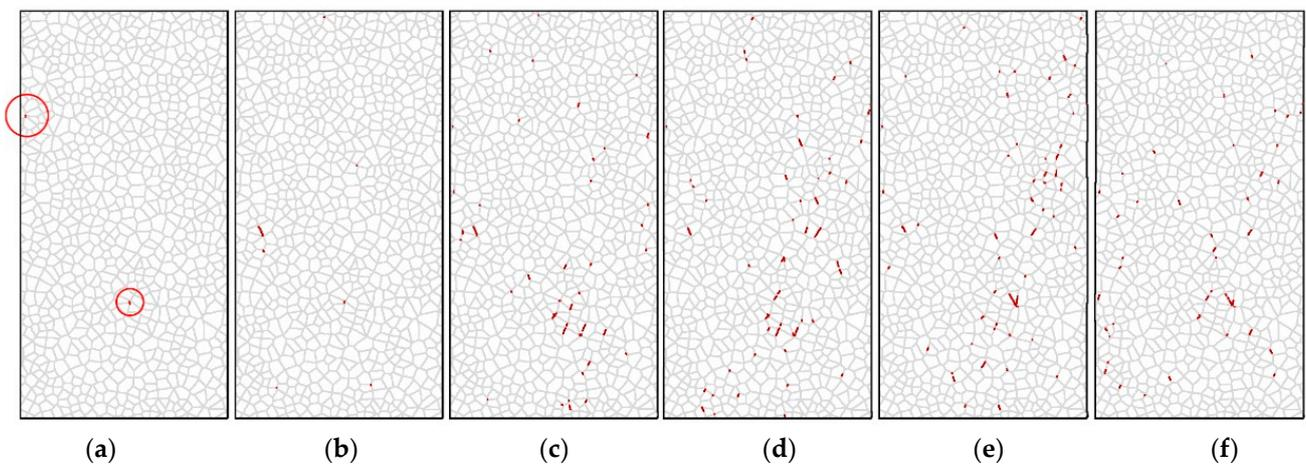
**Figure 9.** Development of shear cracks in rock specimen in UDEC: (a) step 30,000; (b) step 60,000; (c) step 90,000; (d) step 120,000; (e) step 150,000; (f) step 180,000.
