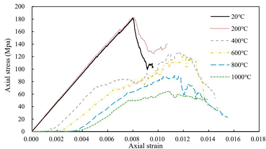
**Figure 6.** Predicted stress-strain relationship for uniaxial compression after calculation of thermal cycle-induced stress.
