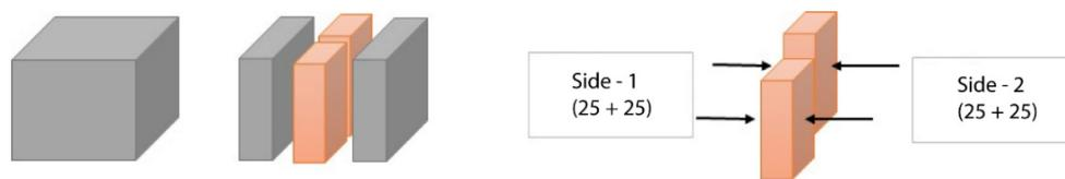
**Figure 2.** Concrete specimen and breakage scheme with sections for pXRF analysis.
