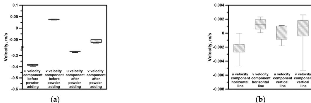
Figure 8. Maximal velocity—Sn in the form of powder: (a) reactor no. 1 with stirring (500 rpm); (b) reactor no. 1 without stirring.
