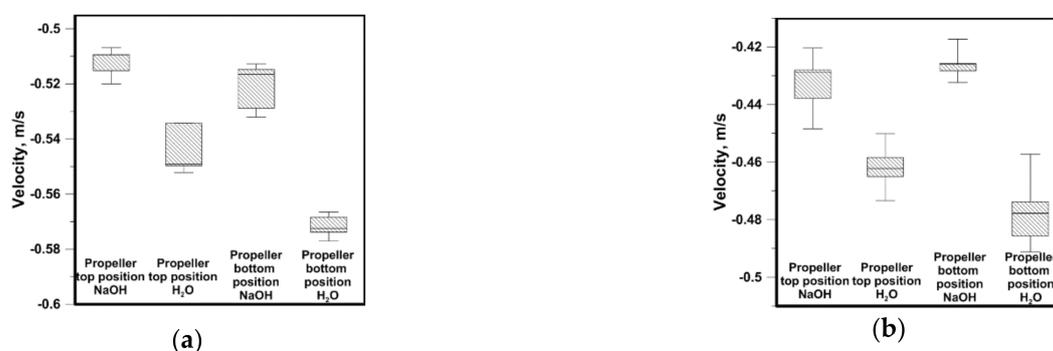
Figure 6. Maximal velocity from horizontal line: (a) reactor no. 1; (b) reactor no. 2.
