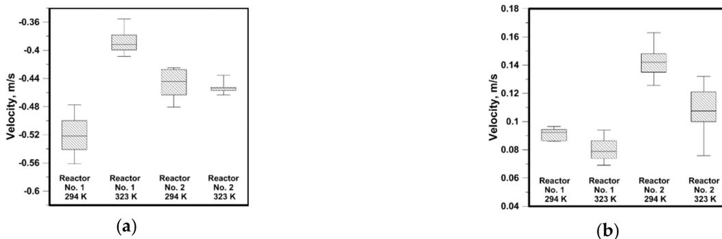
Figure 7. Maximal velocity from the horizontal line—Sn in the form of drops: (a) horizontal component of velocity; (b) vertical component of velocity.
