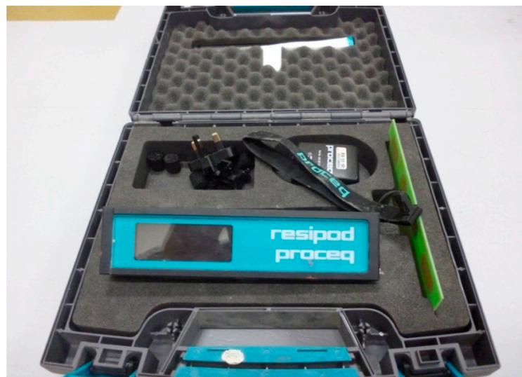
Figure 8. Four-pole resistance measuring instrument.
