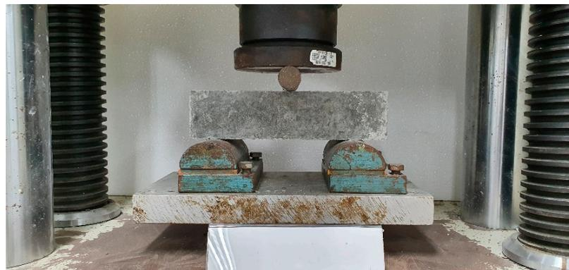
**Figure 4.** Three-point bending test of CFRC setups.
