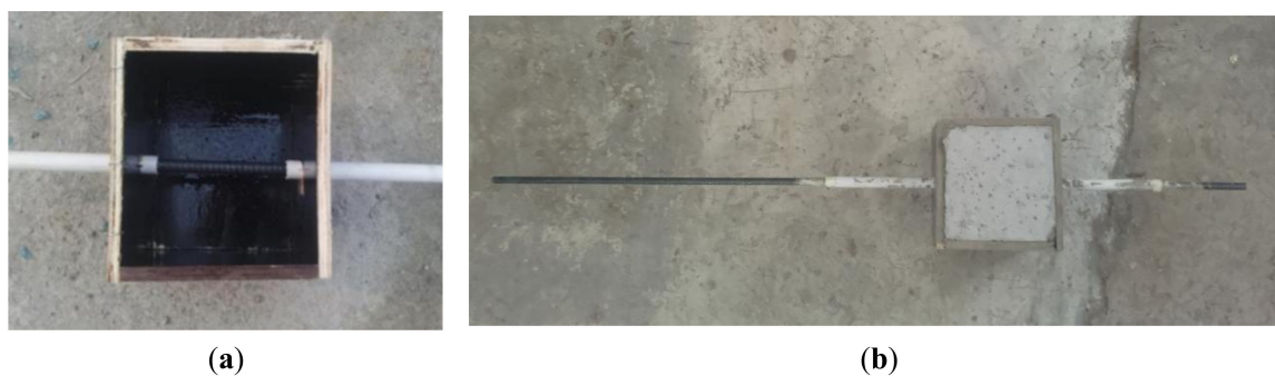
Figure 3. Photograph of the pull-out specimen: (a) mold and (b) cured specimen block.
