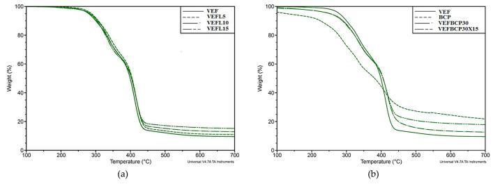
**Figure S1.** TG curves for VEF foams and their composites containing: (a) different amounts of EG L, (b) BCP and a mixture of BCP and EG X.
