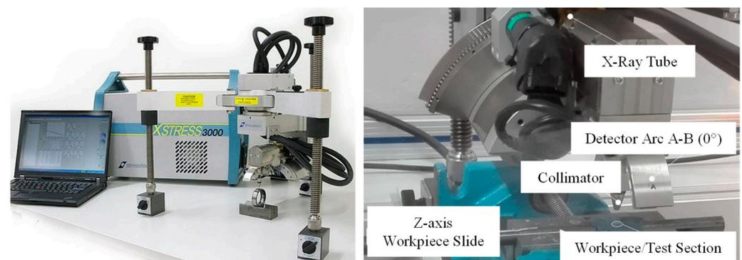
**Figure 3.** XRD analysis—basic system and measurement setup for wire workpiece.
