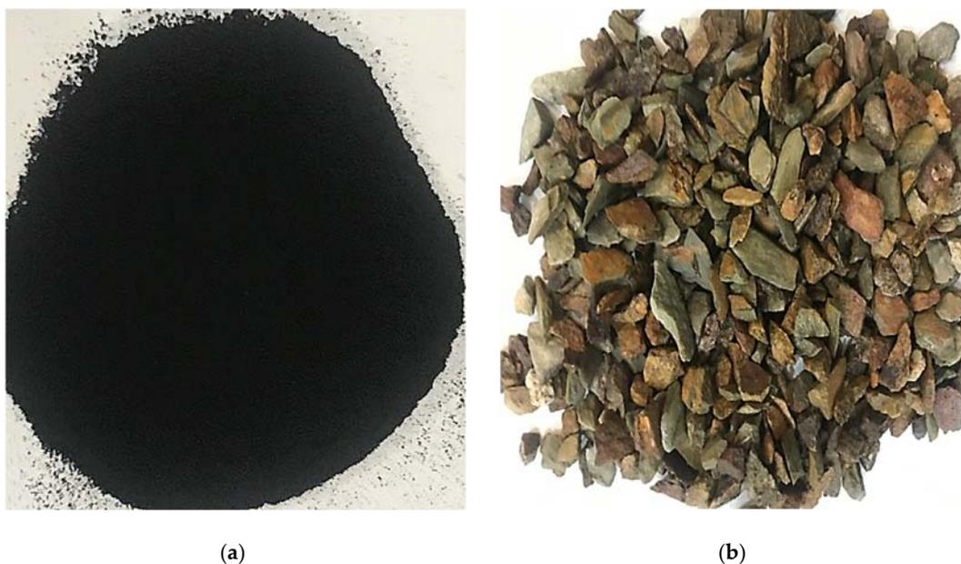
**Figure 1.** Materials used. (a) Recycled rubber waste; (b) Used aggregates.
