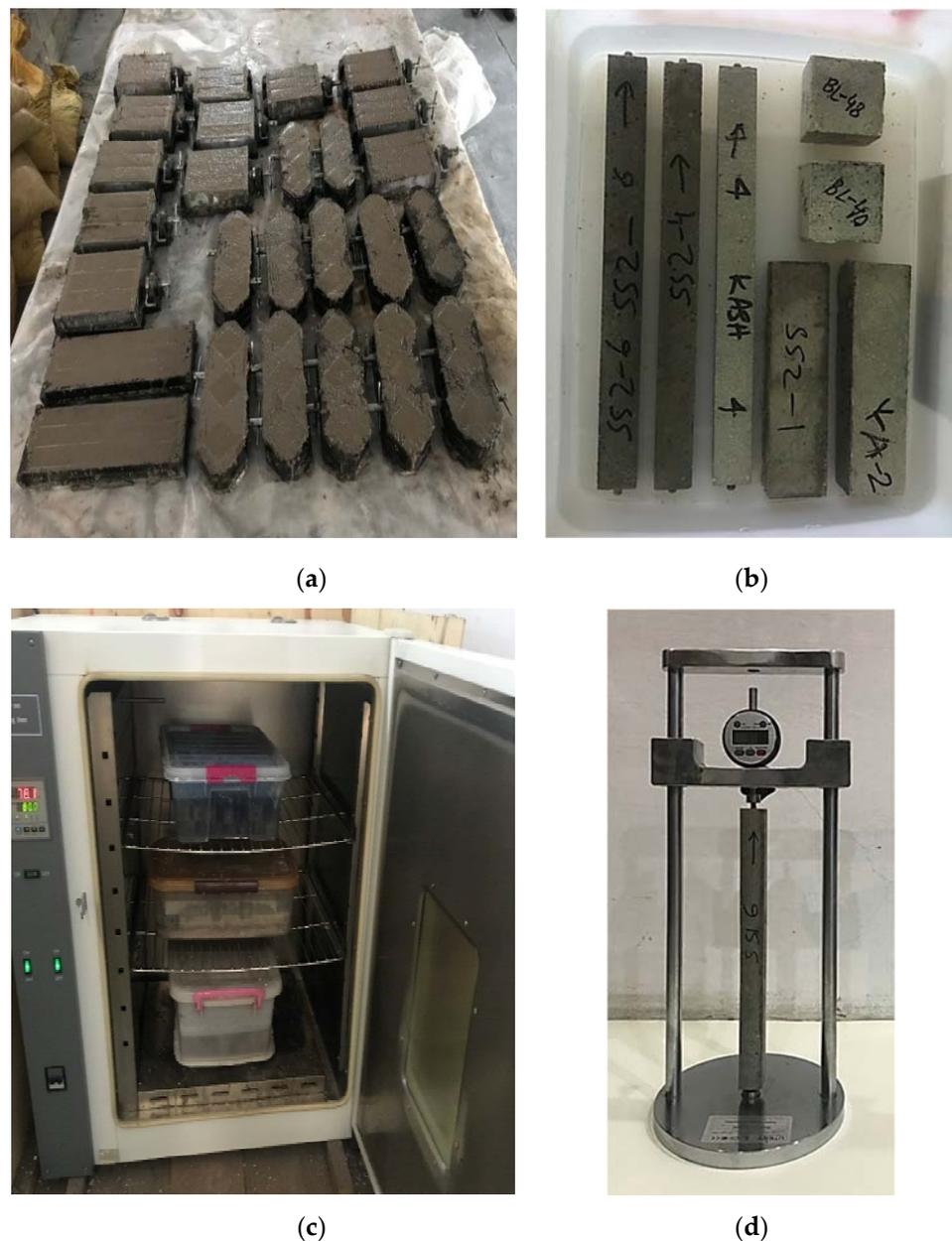
**Figure 2.** Preparation and testing of specimens. (a) Preparation of various specimens; (b) Specimens placed in solution; (c) Specimens placed in oven at 80 °C; (d) Digital length comparator.
