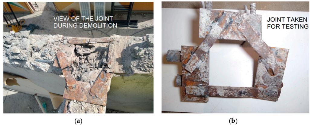
**Figure 13.** Steel joint 3 internal walls: (a) in the process of demolition; and (b) sample taken for testing.
