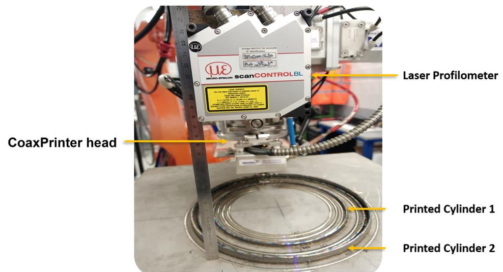
**Figure 7.** Profilometer set-up for data acquisition.
