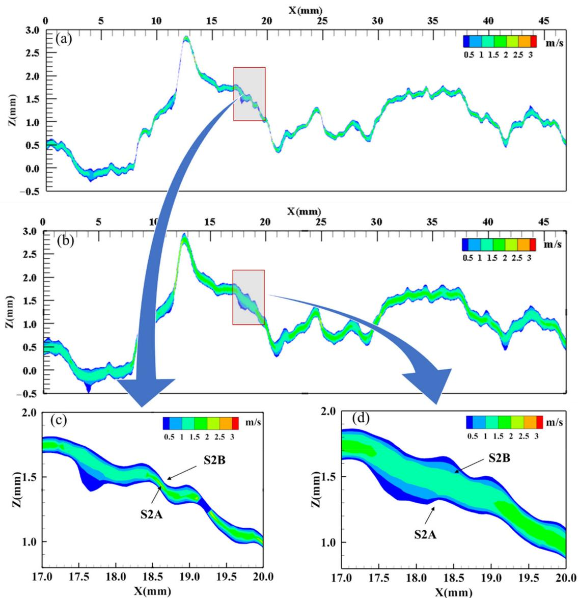
**Figure 17.** Numerical simulation of fluid flow in actual fracture model by Fluent 16.0. (a) Fracture before leaching, (b) fracture after leaching, (c) enlarged view of  $X = 17-20$  mm before leaching and (d) enlarged view of  $X = 17-20$  mm after leaching.
