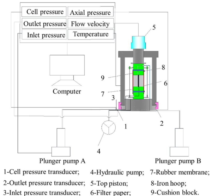
Figure 7. Schematic of experimental setup for permeability experiment.
