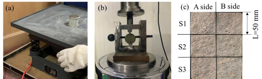
**Figure 3.** Process of samples preparation. (a) Pouring cement samples, (b) Brazilian splitting test and (c) numbering of fracture surfaces.
