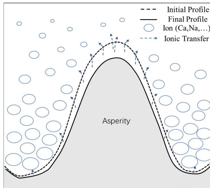
**Figure 20.** Illustration of concrete rough fracture leaching model.
