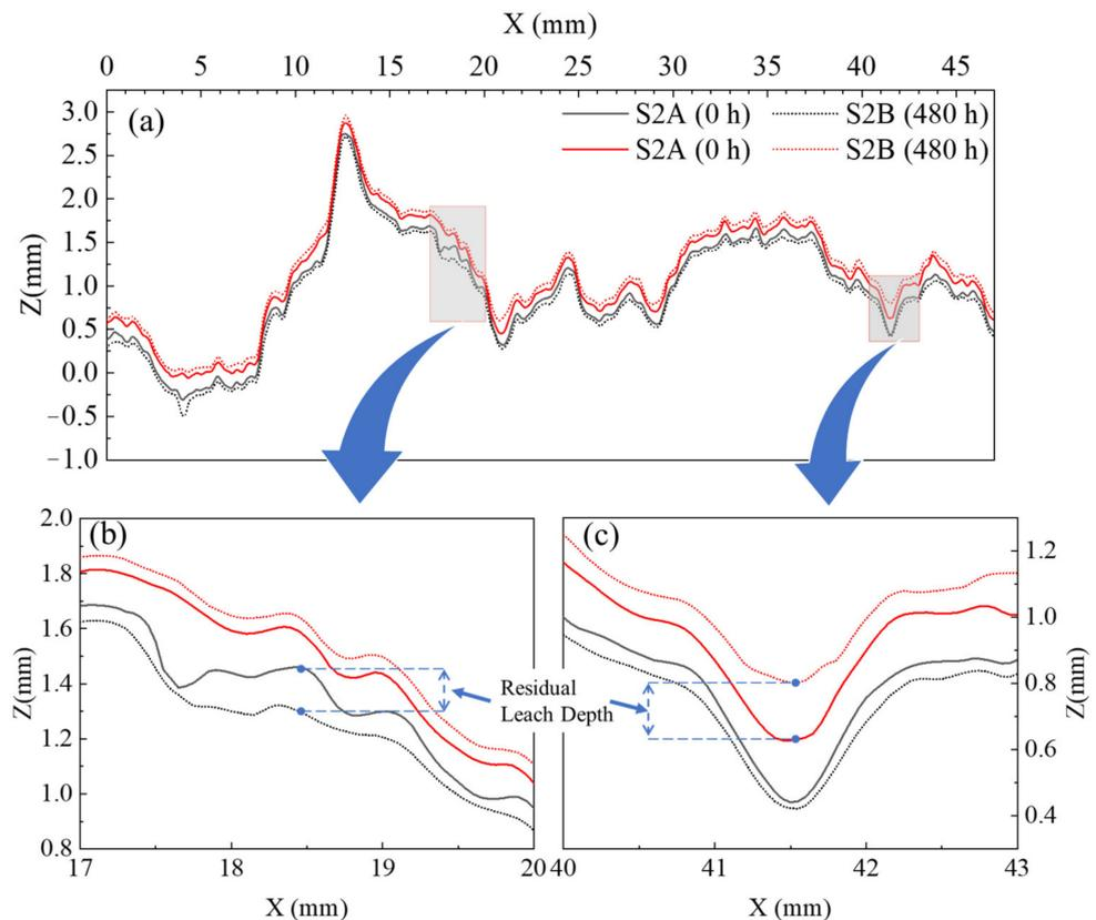
**Figure 14.** Temporal evolutions in profile variation. (a) profile of  $Y = 10$  mm, (b) enlarged view of  $X = 17–20$  mm and (c) enlarged view of  $X = 40–43$  mm.
