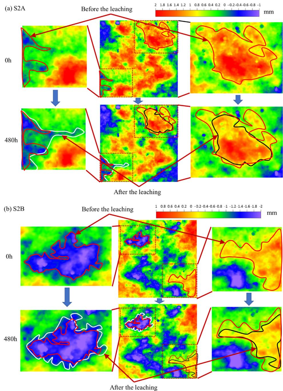
**Figure 9.** Temporal evolution in fracture surface geometry variation.
