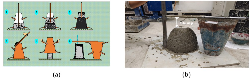
Figure 1. Slump test process, (a) schematic diagram of the slump test operation process, step1: first concrete addition, step2: second concrete addition, step3: third concrete addition, step4: smoothing the mouth of the barrel, step5: demoulding, step6: slump measurement; (b) schematic diagram of slump test measurement.
