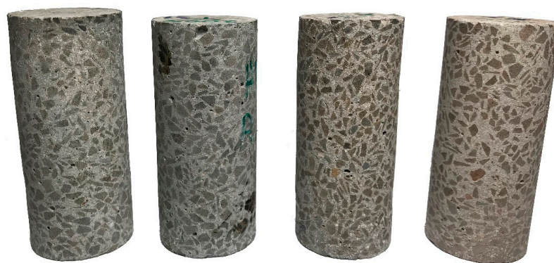
Figure 6. HPFRC 1.1 samples. From left: without heating, 200 °C, 400 °C, 600 °C.
