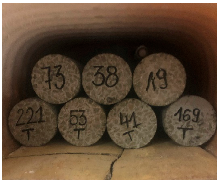
Figure 1. Sample arrangement during heating.
