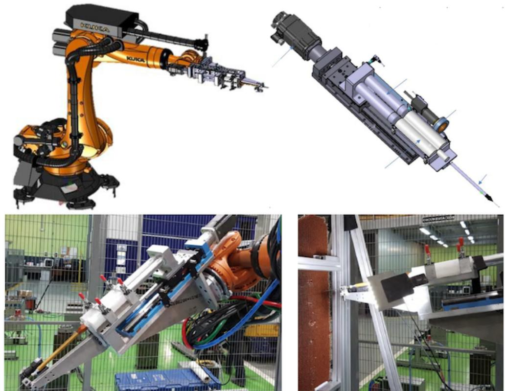
**Figure 6.** The prototype of the single-cell injector. **Upper panels:** Design of the injector group mounted on the linear actuator stage and end-effector mounted on the robotic arm. **Lower panels:** Injection group mounted on a rigid frame fastened to the robot wrist. The injection pipe is supported for rigid guiding. Test for filling the cells of a honeycomb panel.
