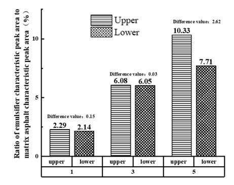
**Figure 11.** Proportion of emulsifier characteristic peak area in upper and lower branch tubes of storage-stabilized tubes.
