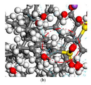
**Figure 7.** Hydrogen bonds between molecules of bio-oil asphalt/water emulsion. (a) Hydrogen bond between water and emulsifier. (b) Hydrogen bond between bio-oil asphalt and emulsifier.
