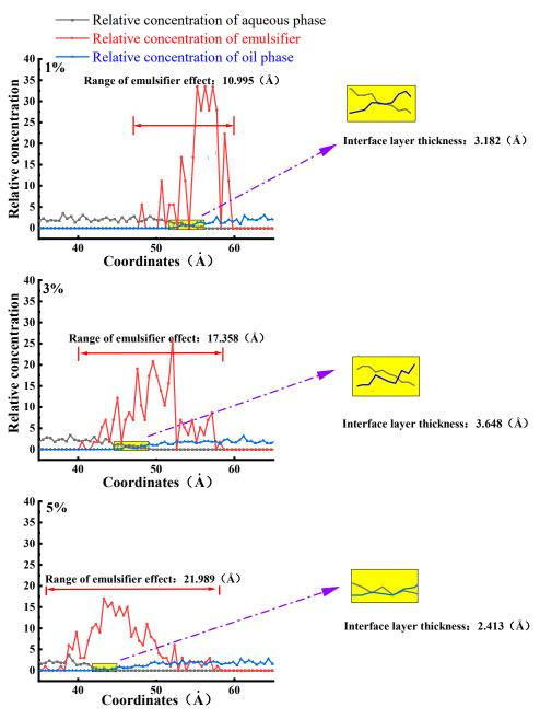
**Figure 6.** Concentration distribution of each component of bio-oil asphalt/water emulsion along the *z*-axis.
