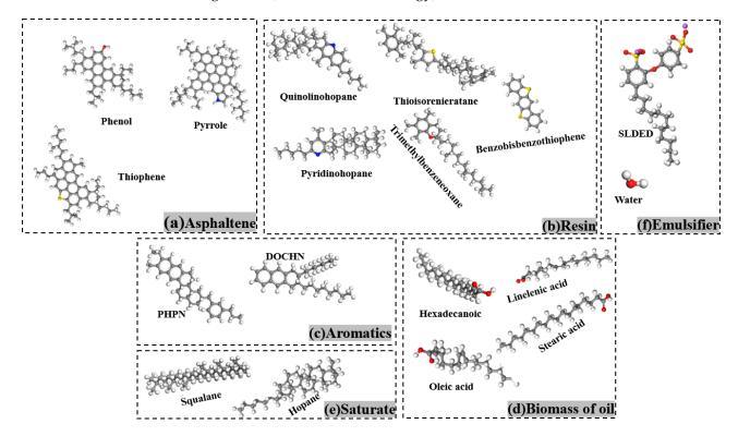
**Figure 1.** Composition diagram of bio-oil asphalt/water emulsion model.
