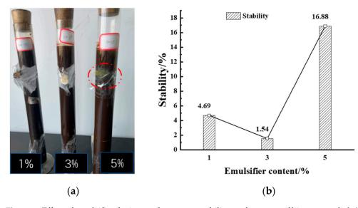
**Figure 9.** Effect of emulsifier dosing on the storage stability performance of biomass asphalt/water emulsion. (a) Flocculation of Asphalt/water emulsion. (b) Stability.
