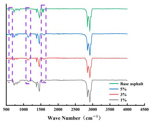
**Figure 2.** Infrared spectra of biomass asphalt/water emulsion with different emulsifier contents (The purple dashed line represents the main characteristic peak changes occurring in the emulsified asphalt relative to the matrix asphalt).
