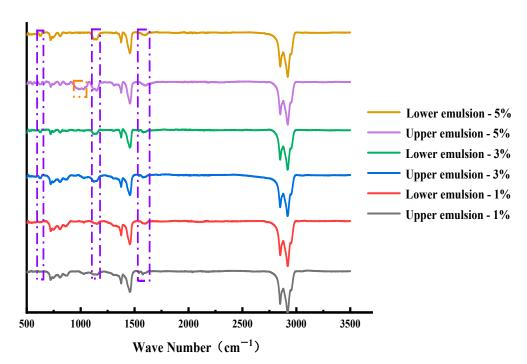
**Figure 10.** Infrared spectra of bio-oil asphalt/water emulsion at different layers with different emulsifier contents (The purple dashed line represents the main characteristic peak changes occurring in the emulsified asphalt relative to the matrix asphalt).
