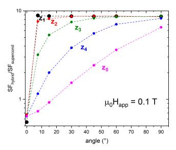
**Figure 11.** Dependence of the ratio between the SFs of the configuration HCC3 and those of the single SC cup,  $SF_{hybrid}/SF_{supercond}$ , on the tilt angle of the applied magnetic field having magnitude 0.1 T. The data refer to the positions  $z_1$  (black dots),  $z_2$  (red dots),  $z_3$  (green dots),  $z_4$  (blue dots), and  $z_5$  (magenta dots).
