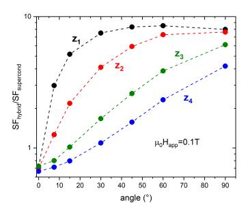
**Figure 8.** Dependence of the ratio between the SFs of the configuration HTC3 and those of the single SC tube,  $SF_{hybrid}/SF_{supercond}$ , on the tilt angle of the applied magnetic field having magnitude 0.1 T. The data refer to positions  $z_1$  (black dots),  $z_2$  (red dots),  $z_3$  (green dots), and  $z_4$  (blue dots).
