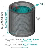
Figure 9. Schematic view of the hybrid layout HCC3 consisting of two SC/FM superimposed cups with the FM cup protruding above the SC one. The shield sizes are reported in the picture, where  $R_o$  and  $R_i$  are the outer and inner radii of the cup layouts, respectively; the base thickness of the SC cup is 4.20 mm, while base thickness of the FM cup is 2.50 mm;  $\Delta h = 3.5$  mm represents the height difference between the cup edges.
