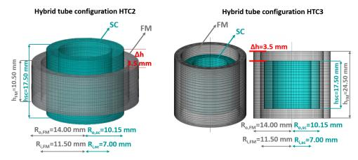
**Figure 4.** Schematic view of the tubular hybrid layouts consisting in SC/FM superimposed tubes with the SC tube protruding above the FM one (HTC2) and in SC/FM superimposed tubes with the FM tube protruding above the SC one (HTC3). The shield sizes are reported in the picture, where  $R_o$  and  $R_i$  are the outer and inner radii of the tubular layouts, respectively;  $\Delta h$  represents the height difference between the tubes edges.
