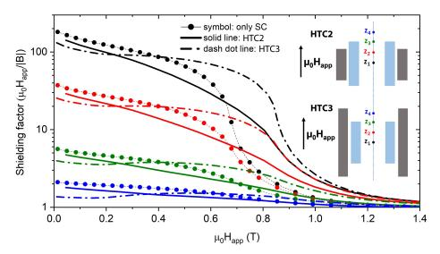
**Figure 6.** Comparison between the SFs of the single SC tube and of the configurations HTC2 and HTC3 in the AF mode. Assuming (x,y,z) = (0,0,0) the coordinate of the tube center, the plotted curves were calculated at the z values:  $z_1 = 0$  mm,  $z_2 = 4.4$  mm,  $z_3 = 8.8$  mm (SC shield edge coordinate), and  $z_4 = 13.1$  mm.
