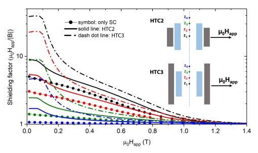
**Figure 5.** Comparison between the SFs of the single SC tube and of the HTC2 and HTC3 configurations in the TF mode. Assuming (x,y,z) = (0,0,0) the coordinate of the tube center, the plotted curves were calculated at the z values:  $z_1 = 0$  mm,  $z_2 = 4.4$  mm,  $z_3 = 8.8$  mm (SC shield edge coordinate) and  $z_4 = 12$  mm.
