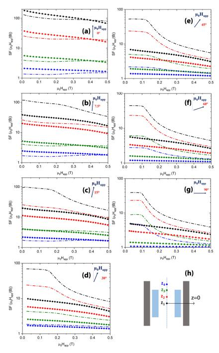
**Figure 7.** Comparison between the SFs of the single SC tube (dot symbols) and the configuration HTC3 (dash dot lines). Each frame (**a**–**g**) corresponds to a different tilt angle of the applied magnetic field. Assuming z = 0, the axial coordinate of the tube center, the curves refer to positions  $z_1 = 0$  mm (black curves),  $z_2 = 4.4$  mm (red curves),  $z_3 = 8.8$  mm (green curves), and  $z_4 = 13.1$  mm (blue curves), indicated in the HTC3 schematic view shown in the frame (**h**).
