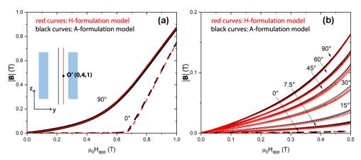
**Figure 3.** Comparison between the magnetic flux density values calculated at point O' (whose coordinates related to point O are (0 mm, 4 mm, 1 mm), i.e., 4 mm away from the tube center along the radial direction and 1 mm away along the axial one), using the **H**-formulation (red curves) and the **A**-formulation (black curves). Calculations were carried out in the axial and transverse field orientations (**a**) and for different angles of the applied field (**b**).
