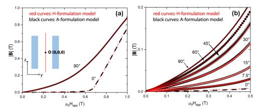
**Figure 2.** Comparison between the magnetic flux density values calculated in the tube center O (whose coordinates were set to (0,0,0)) of the tubular shield shown in Figure 1 using the **H**-formulation (red curves) and the **A**-formulation (black curves). Calculations were carried out in the axial and transverse field orientations (**a**) and for different angles of the applied field (**b**).
