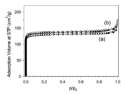
**Figure 5.** The  $N_2$  adsorption and desorption isotherms of NaX zeolites synthesized by: (**a**) magnetic induction heating; (**b**) convection oil bath heating. (Closed symbol: adsorption; open symbol: desorption).
