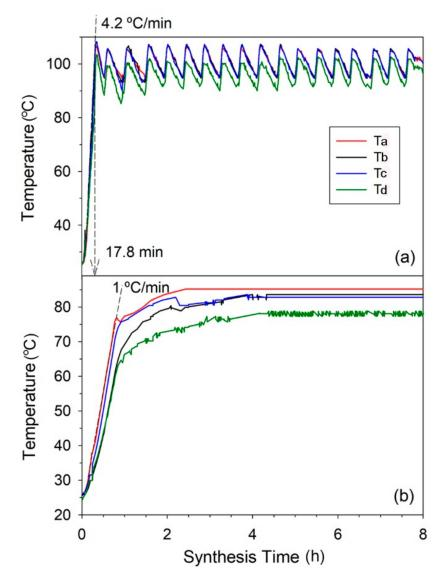
**Figure 2.** The temperature profiles of the reaction mixture of NaX zeolite for non-stirred synthesis by: (a) magnetic induction heating; (b) convection oil bath heating.
