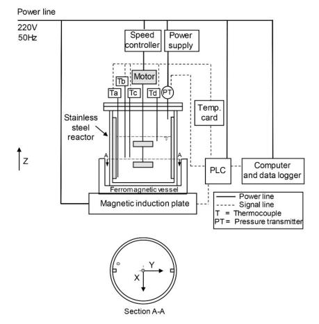
Figure 1. The bench-scale reactor setup with the magnetic induction heating plate.
