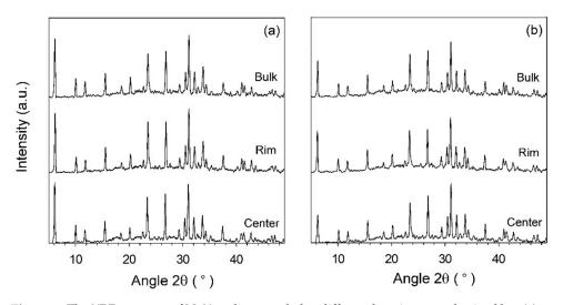
**Figure 3.** The XRD patterns of NaX zeolite sampled at different locations, synthesized by: (**a**) magnetic induction heating; (**b**) convection oil bath heating.
