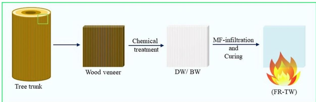
**Figure 37.** Schematic illustration of fire-retardant transparent wood (FR-TW) fabrication based on melamine formaldehyde, MF. DW is delignified wood where most lignin is removed, and BW is bleached wood where lignin chromophores are modified and a small amount of lignin removed. Reprinted from [50] under CC-BY license.
