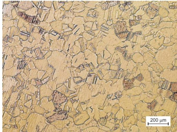
**Figure 3.** Initial microstructure of CuZn36 (% at.) alloy.
