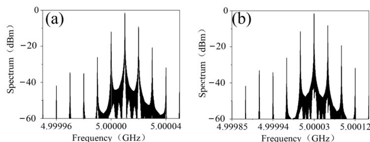
**Figure 4.** The simulated spectrum of the frequency-mixed transmitted EM wave biased with (a) 10 kHz and (b) 30 kHz upper triangle voltage signal.
