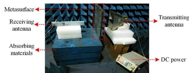
**Figure 2.** Diagram of transmission measurement of the active metasurface.
