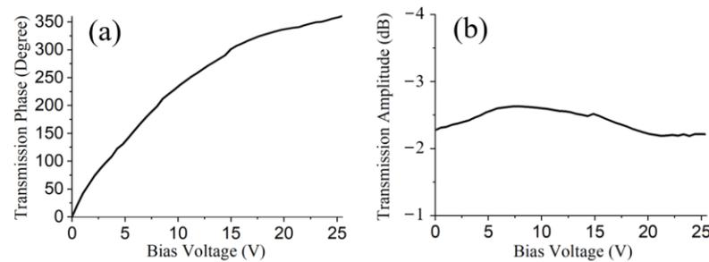
**Figure 3.** Transmission phase (a) and transmission amplitude (b) of the metasurface at 5 GHz versus bias voltage.
