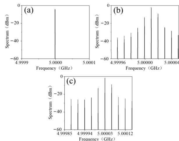
**Figure 6.** The measured spectrum of the frequency-mixed transmitted EM wave with (a) no voltage biasing and with (b) 10 kHz or (c) 30 kHz upper triangle voltage signal.
