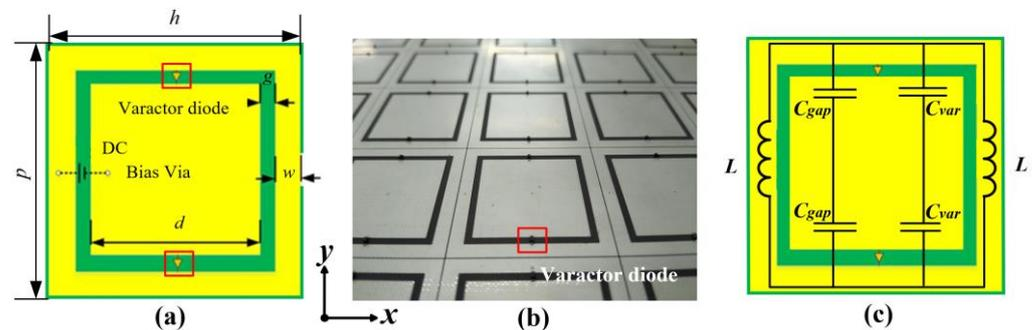
**Figure 1.** (a) Geometry of the unit cell. (b) The fabricated active metasurface sample. (c) Equivalent circuit of the unit cell.
