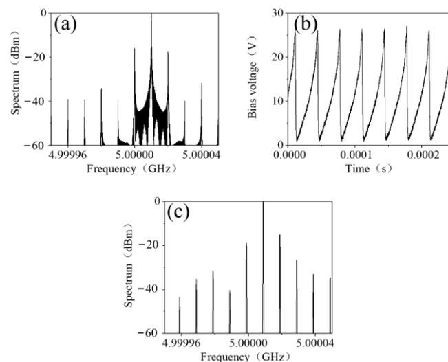
**Figure 7.** (a) The simulated spectrum of the frequency-mixed transmitted EM wave biased with a 10 kHz voltage waveform  $v_b(t)$ , (b) a 10 kHz voltage waveform  $v_b(t)$  and (c) the measured spectrum of the frequency-mixed transmitted EM wave biased with a 10 kHz voltage waveform  $v_b(t)$ .
