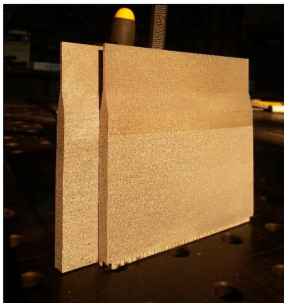
**Figure 1.** Test plates made by the SLM method ready for welding.
