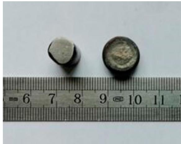
**Figure 5.** Samples after canning and isothermal compression.
