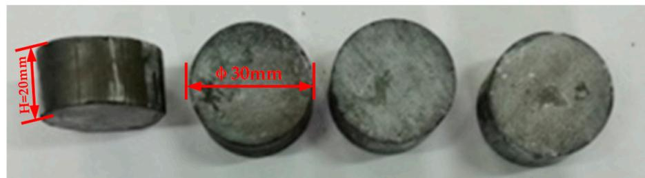
**Figure 4.** Sintered Zr-6Al-0.1B alloy workpieces.
