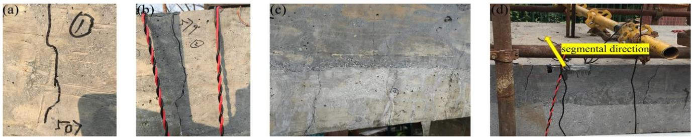
**Figure 7.** Development of cracks at the beginning of the test: (a) the first crack when the load was increased to 507 kN; (b) the crack when loaded to 579 kN; (c) cracks in midspan tensile zone when the load reached 650 kN; and (d) cracks in bottom plate developing along segments when loaded to 650 kN.
