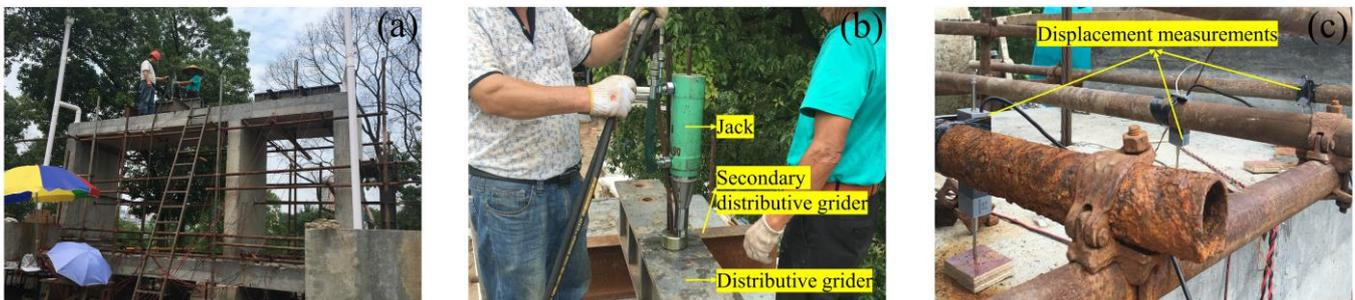
Figure 5. On-site loading of the prefabricated utility tunnel: (a) full-scale utility tunnel; (b) jack; and (c) displacement measurements.
