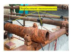
**Figure 5.** On-site loading of the prefabricated utility tunnel: (a) full-scale utility tunnel; (b) jack; and (c) displacement measurements.
