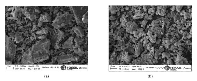
Figure 3. Industrial waste morphology: (a) ORPS and (b) CCS.
