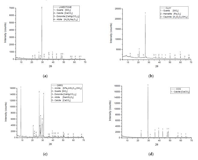
Figure 4. Mineral characterization of the raw materials. Limestone (a), Clay (b), ORPS (c), and CCS (d).
