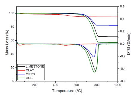
Figure 6. Thermogravimetric analyses of the raw materials.
