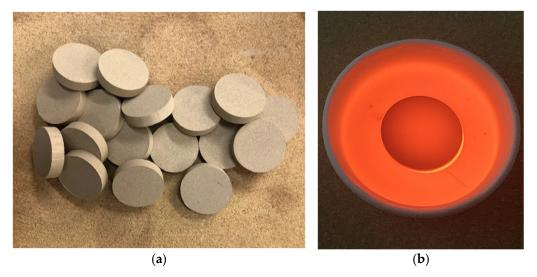
Figure 1. Tablet samples: (a) after pressing and (b) after clinkering.
