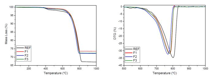
Figure 7. Thermogravimetric analysis of the raw clinker mixtures.
