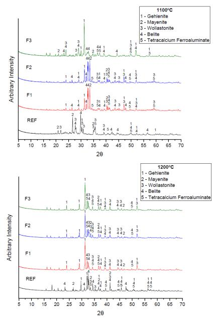
Figure 5. Mineral analysis of experimental clinkers produced.
