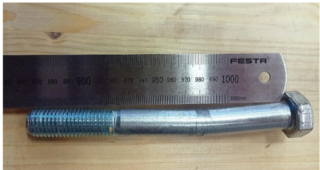
**Figure 24.** Deformed bolt after the experimental testing.
