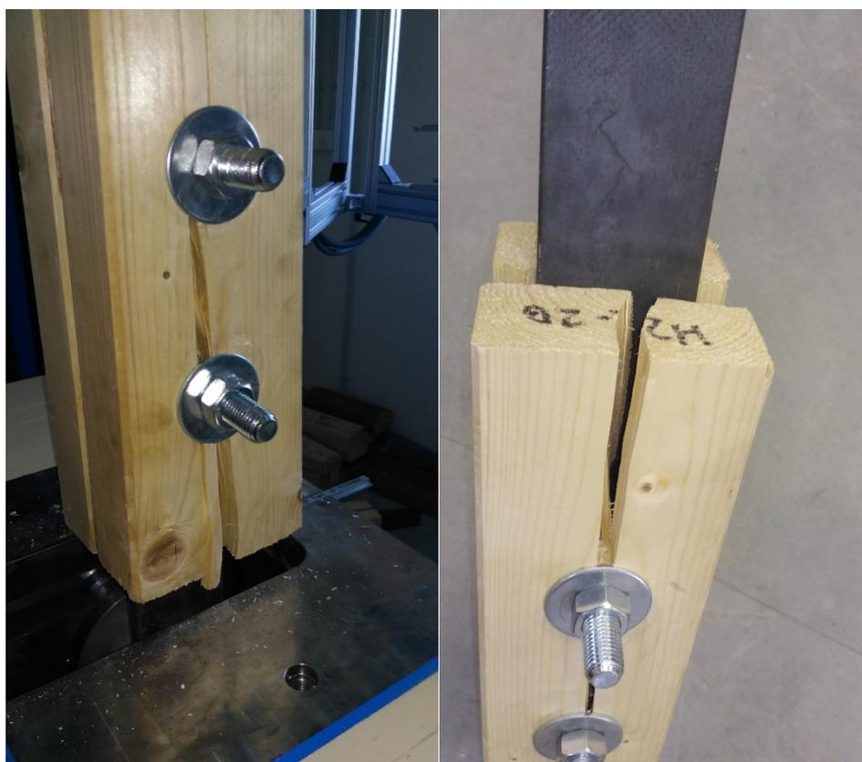
**Figure 19.** Specimens of squared timber connections after failure.
