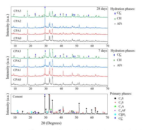
**Figure 2.** X-ray diffraction patterns for cement (no hydration) and CPA samples after hydration at 7 days and 28 days together with the identified crystalline phases: Alite (C<sub>3</sub>S), belite (C<sub>2</sub>S), gypsum (C<u>S</u>), tricalcium aluminate (C<sub>3</sub>A) and aluminoferite (C<sub>4</sub>AF). Hydration compounds: Portlandite (CH), calcite (C<u>C</u>), and ettringite (AFt).
