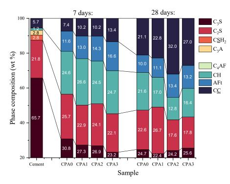
**Figure 3.** Results of the quantitative crystalline phase analysis using the XRD patterns for cement and CPA composites after hydration at 7 and 28 days.
