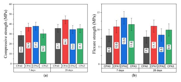
**Figure 4.** Mechanical properties of CPA samples at 7 and 28 days: (**a**) Compressive strength and (**b**) flexural strength.
