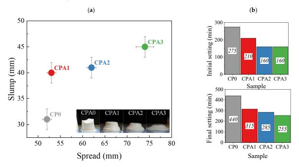
**Figure 1.** Fresh CPA paste properties: (**a**) Mini-slump tests giving the average height and spread of the casted cement samples (see inset) and (**b**) initial and final setting times determined using the Vicat needle test.
