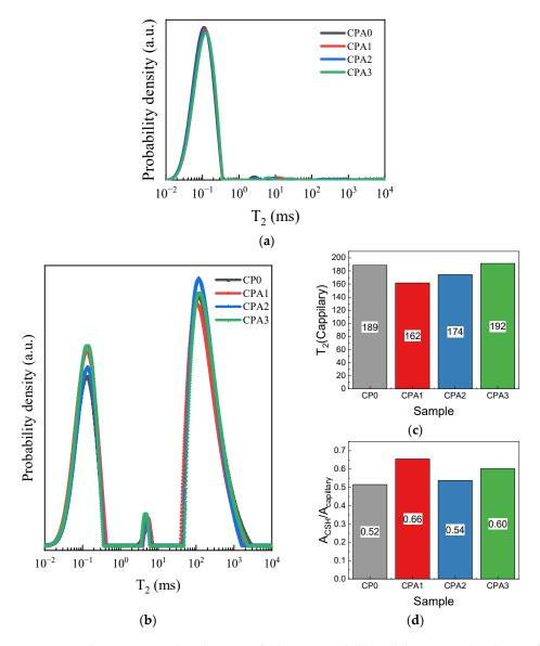
**Figure 7.** Relaxation time distributions of (**a**) water and (**b**) cyclohexane molecules confined in hardened CPA samples, followed by parameters extracted from the distribution of cyclohexane: (**c**) The center of the  $T_2$  relaxation peak for capillary pores and (**d**) the ratio between the areas of the intra C-S-H peak (at  $T_2 \sim 10^{-1}$  ms) and the capillary peak.
