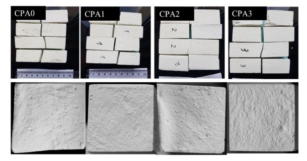
**Figure 5.** Visual inspection of CPA samples after flexure tests at 28 days, revealing textural changes of the flexure plane associated with variations in accelerator concentration.
