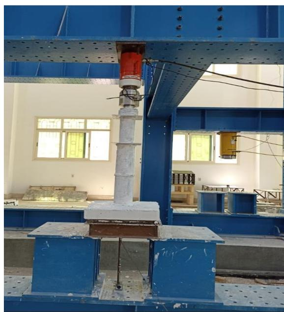
(a) Experimental load setup
