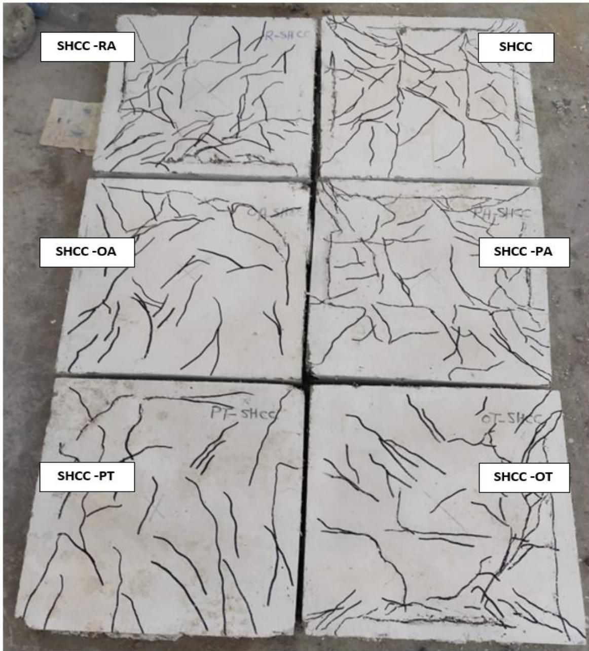
Figure 9. SHCC specimens cracks.
