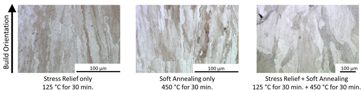
Figure 8. Microstructure of heat treated samples, the arrow indicates the build direction.
